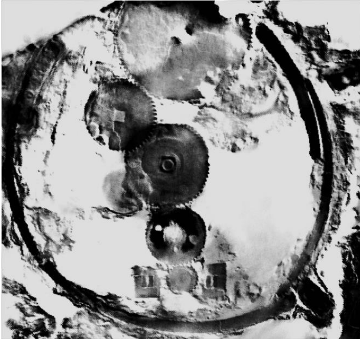
Figure 32 CT scan of the Mechanism. Gears and arc like blades can be seen, that protect the gears from breaking as they rotate and deform from the torque.
