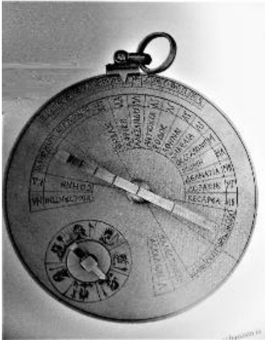
Byzantine period ancient sundial calendar mechanism (around 500 AD) worked by gears. Programmed to work for various latitudes and cities (Alexandria, Antioch, Rhodes, Athens, Sicily, Thessaly, Rome, Dalmatia, Caesarea). Reconstruction of Dionysis Kriaris. The original is at the Science Museum London.
