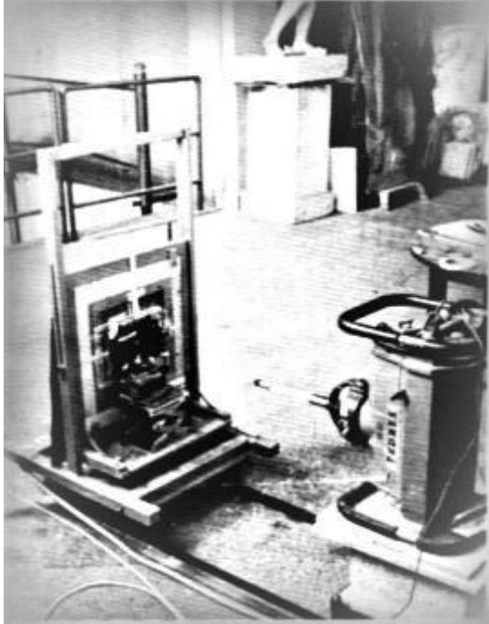
Image of ray device made by Democritus' nuclear physicist Char. Caracalos and obtained stereoscopic images of the Mechanism with which Derek de Solla Price made the study of the Mechanism with counts of the teeth of the gears by Emilia wife of Caracalos.
