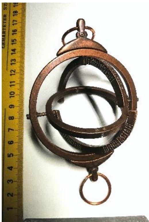
Figure 83 A portable solar clock and mini astrolabe, 23-24 centuries ago from Greece. Suitable to be used in many cities and at all latitudes. Construction by Mr Dionysis Kriaris
