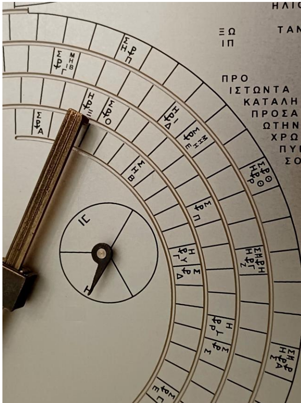
Figure 23 Part of the eclipse dial. It shows in every month if there is a lunar ( \Sigma ) or solar ( H ) eclipse. It shows the hour of the eclipse. The small circular dial shows how many hours (8 or 16) to add the hour indicated in case of the second or third Saros cycle.
