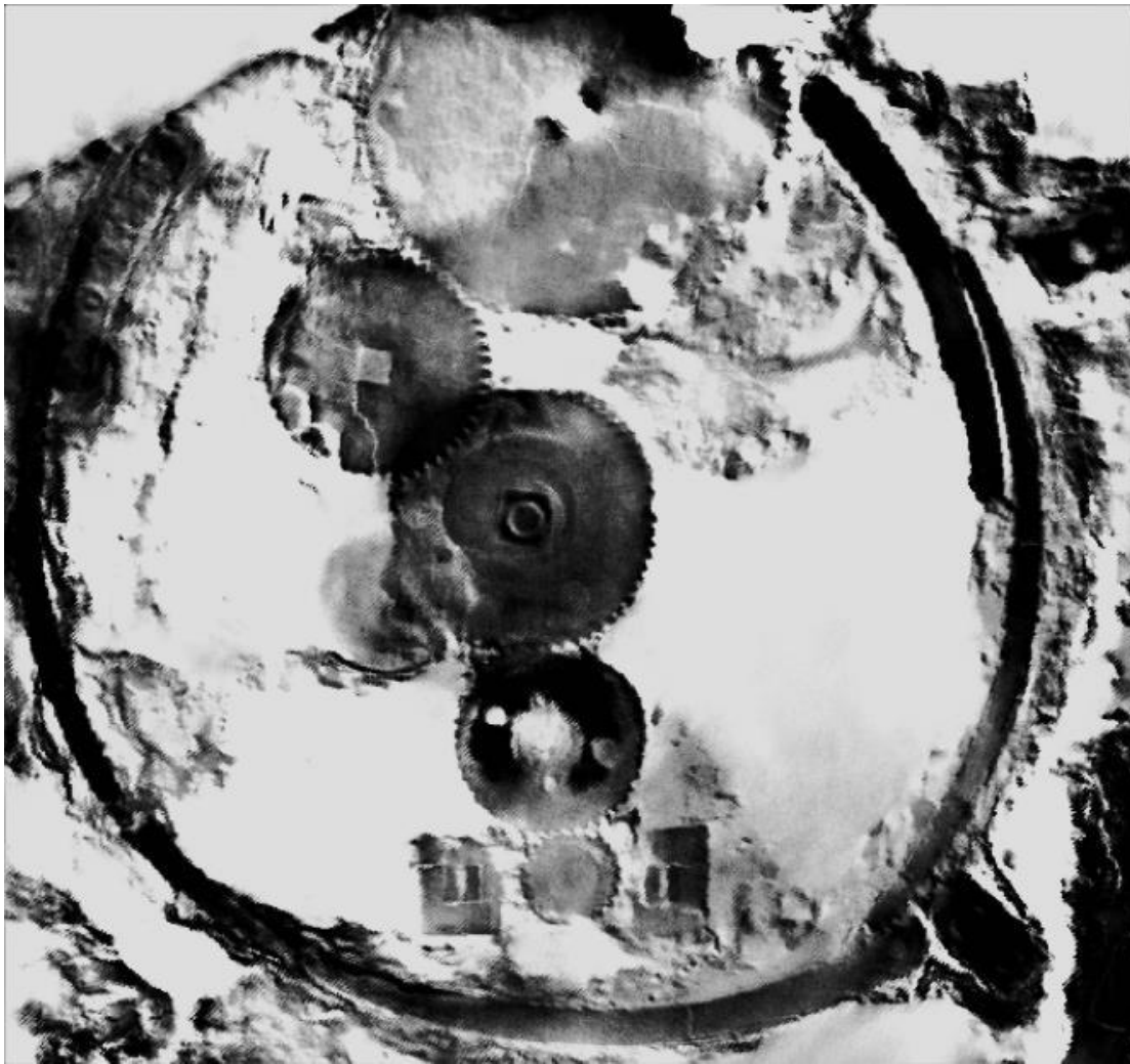
CT scan of the Mechanism. Gears and the 'safes', arched plates that protect the gears from breaking as they rotate and deform under the strain of the torque that turns the gears, can be seen.
