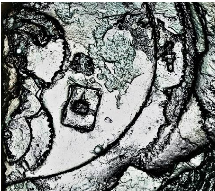
Figure 21 Two of the four gears (left) that make the moon to move following Kepler's second law using the epicyclical theory. The four gears add two circular motions. This image is made using the PTM method of Dr. T. Malzbender (HP) using
