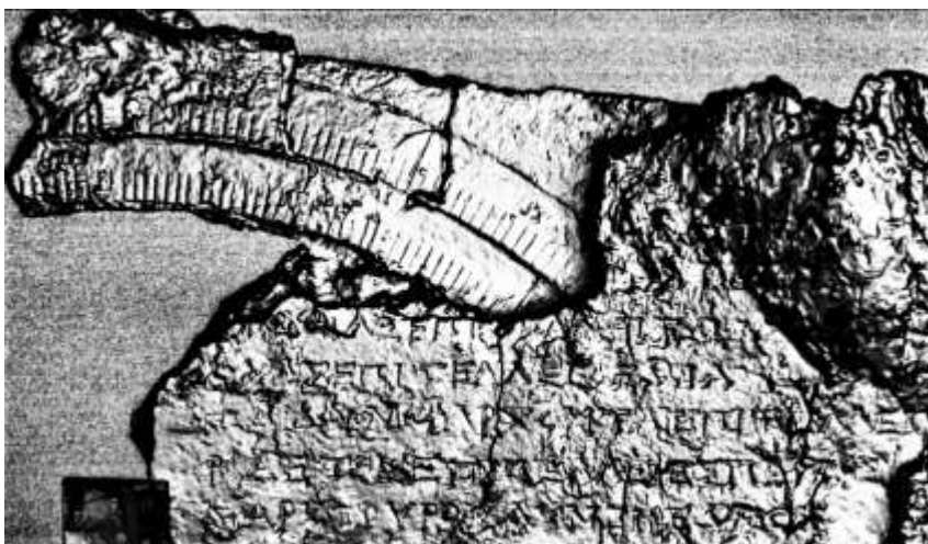
Figure 7. Fragment C, scales and part of the PARAPEGMA. Part of the scale of the year and the scale of the zodiac.
