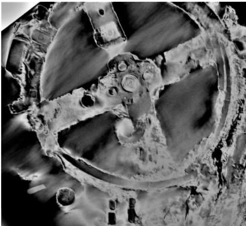
Figure 2 Computer tomography of the largest gear, the gear of the Sun
