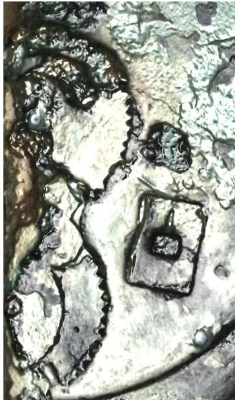
Two gears of the four that make the lunar trajectory to follow Kepler's second law
