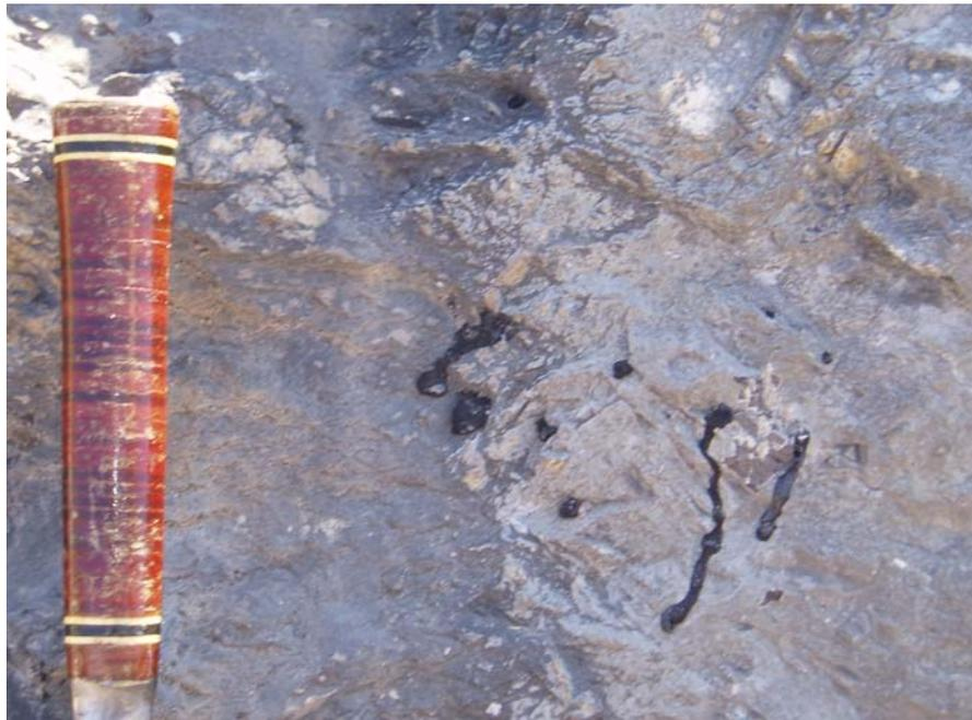
**Fig. 16** Eocene limestone impregnated with oil
