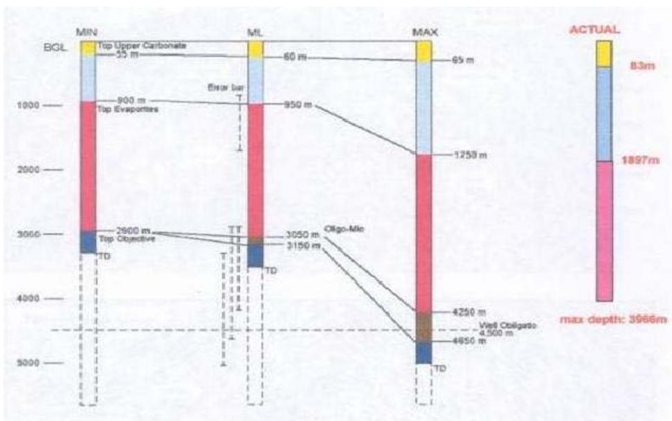
**Fig. 34** Well Demetra-1: Pre-drill prognosis vs. actual drilled section
