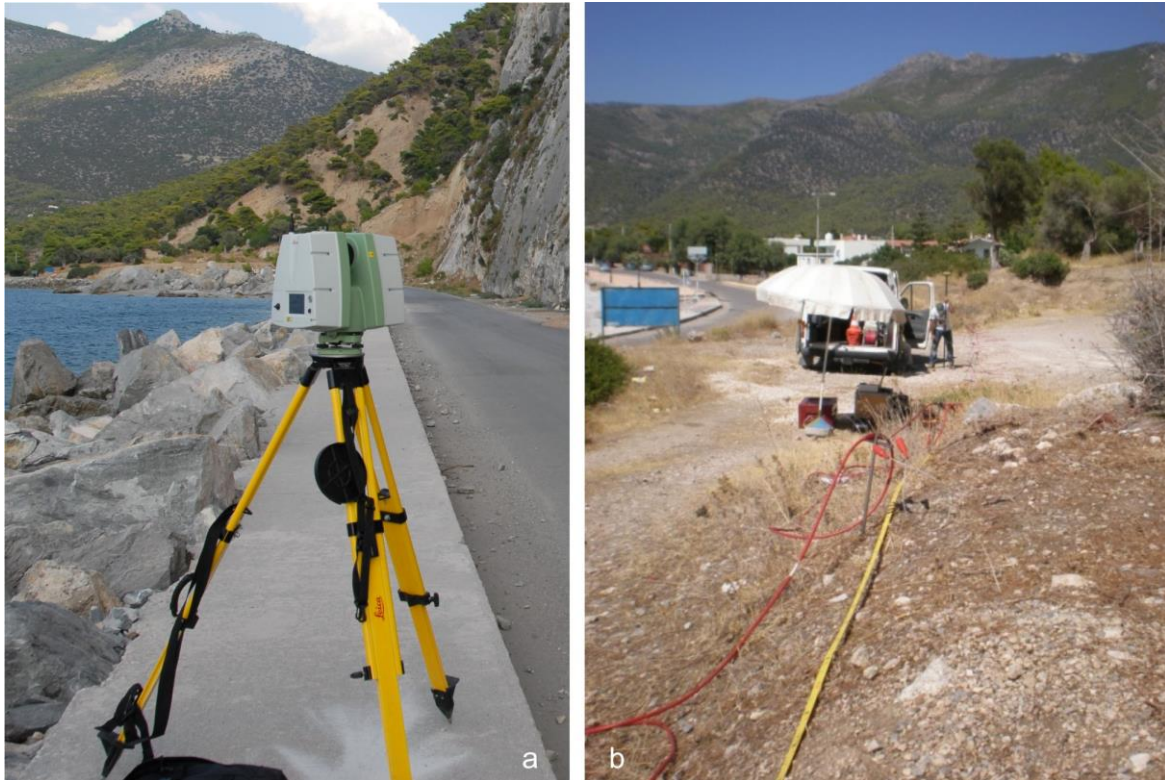
Figure 3. Field work data acquisition by surveying with the terrestrial laser scanner at the station SG-2 (a) and geophysical tomography along the ERT-1 section (b).
