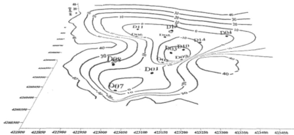
Figure 5. 3D representation of the geoelectrical basement (limestones / dolomites).
