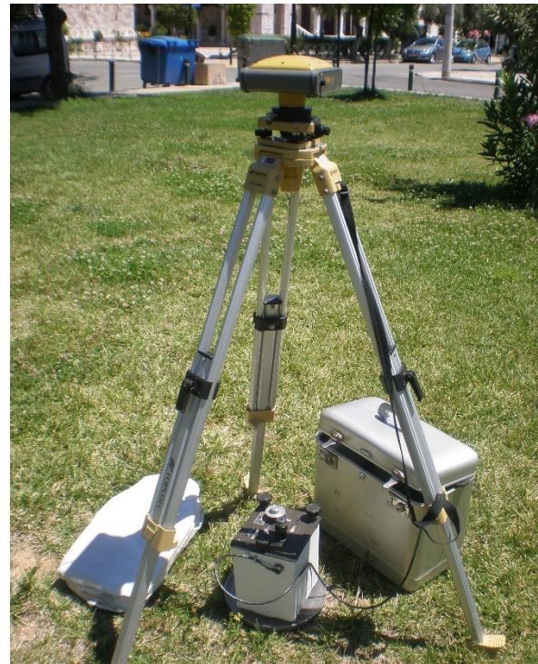
Figure 4.8: Development of the gravimeter and dGPS TopCon HiperPro antenna (placed on the tripod over the gravimeter) at the field.
