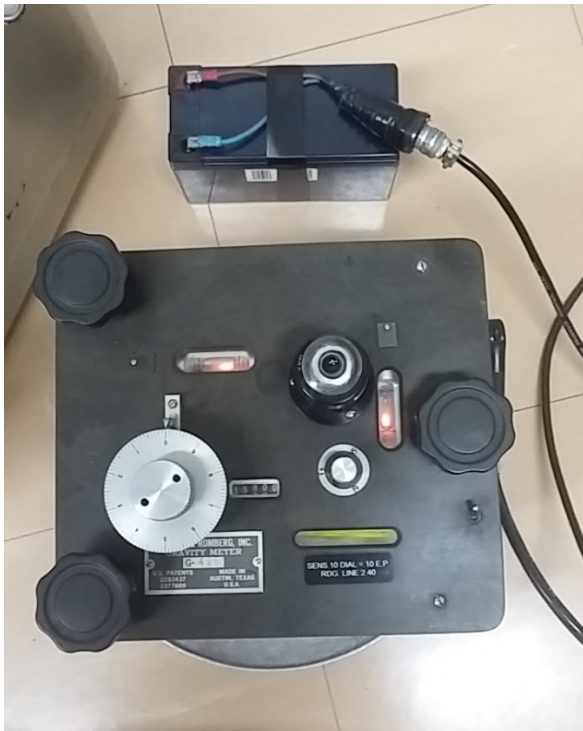
Figure 4.7: The gravimeter LaCoste & Romberg G-496 , placed the concave plate.
