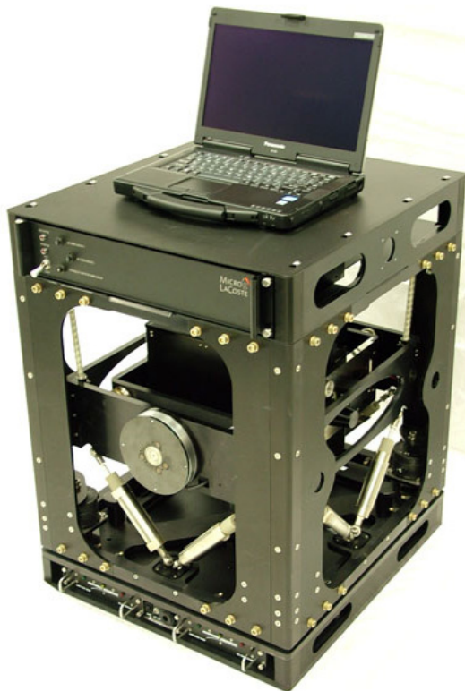
Figure 3.11: The MGS-6 Gravity Meter on gyro stabilized platform
