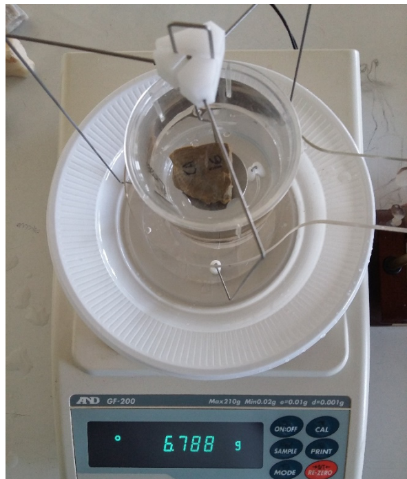
Figure 4.12: Weighing the saturated specimen dipped in water ( W_3 ) with the aid of special kit.
