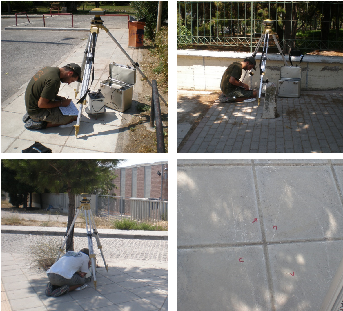
Figures 4.2: Some of the established local gravity bases. Top left: “Rouf”, Top right: “Filadelfia”, Bottom left: “Vrilissia”. The bottom right photograph illustrates the permanent marks of a base.
