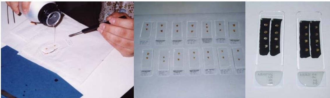
**Figure 9.2.3.** Distribution of resin over the spine sections, air-drying and spine cuts embedded in resin and mounted with Eukitt.
