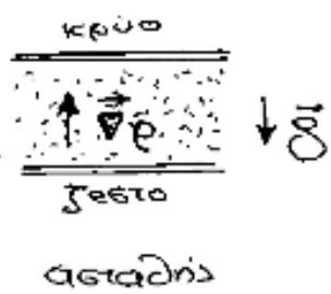
$$\left. \begin{array}{l} \vec{\nabla}_\rho \times \vec{\nabla}_\phi = 0 \\ \vec{\nabla}_\phi = -\vec{g} \end{array} \right\} \vec{\nabla}_\rho \parallel \vec{g}$$
