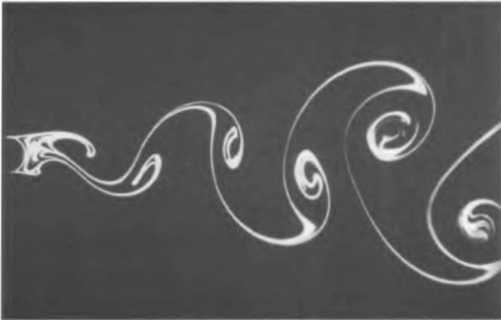
Fig. 1.6. Kármán vortex street behind a circular cylinder at R = 140 (Van Dyke 1982). Photograph S. Taneda.
