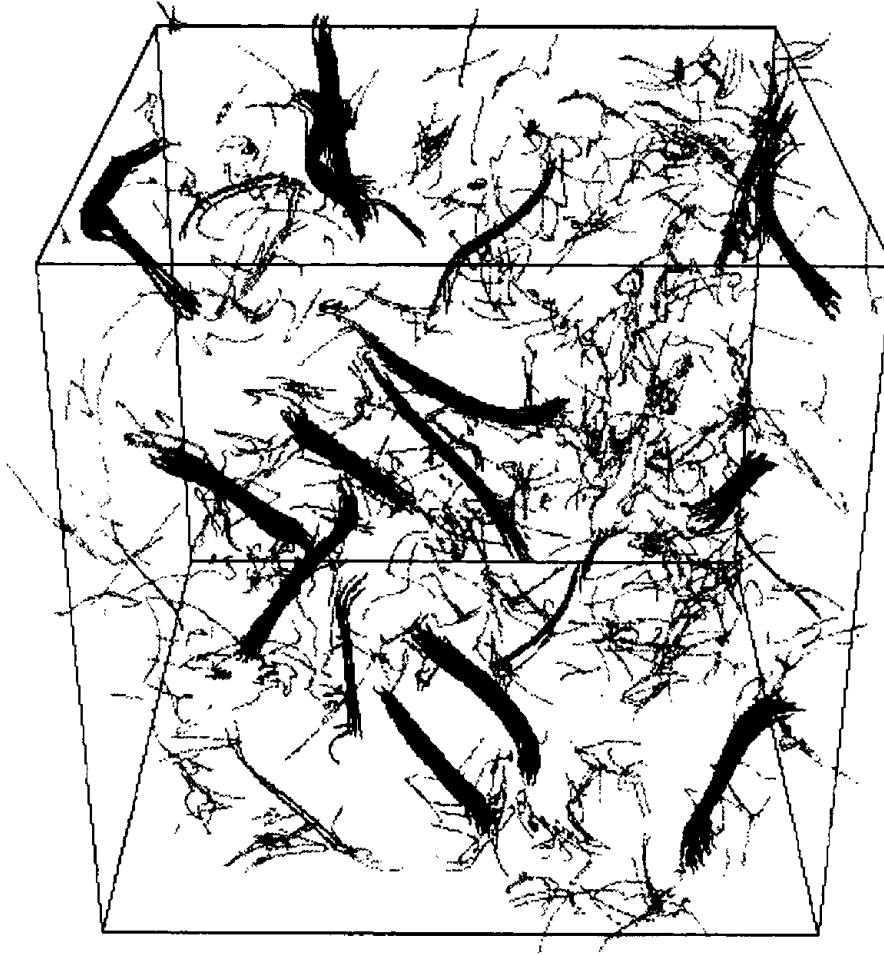
Fig. 7.4. Intermittent vortex filaments in a three-dimensional turbulent fluid simulated on a computer (She, Jackson and Orszag 1991).
