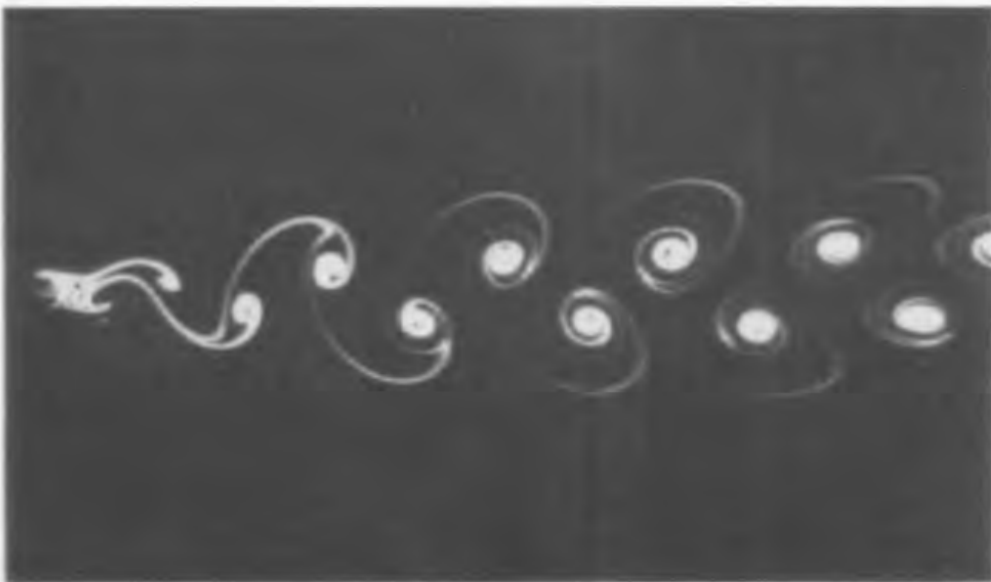
Fig. 1.7. Kármán vortex street behind a circular cylinder at R = 105 (Van Dyke 1982). Photograph S. Taneda.
