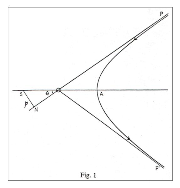
on escaping the atom is OP'. OP and OP' make equal angles with the line SA, where A is the apse of the hyperbola. p = SN = P perpendicular distance from centre on direction of initial motion of particle.
