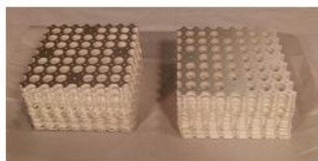
FIGURE 3.6: Picture of the horn array, produced for the technological demonstrator of QUBIC (left). Close picture of a horn cut (center). Mirror, produced for the technological demonstrator (right).
