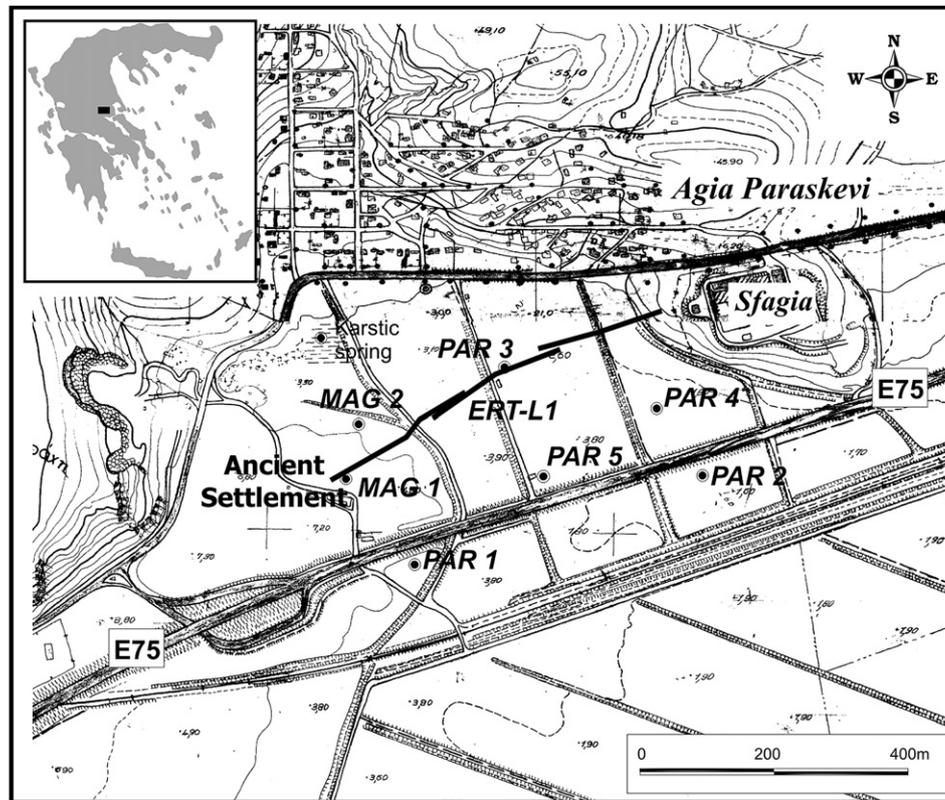
Fig. 2. Site map of Agia Paraskevi area, including the Prehistoric settlement, where the locations of the boreholes and the lines of the electrical resistivity tomography are shown. E75 is the Athens-Thessaloniki national highway.
