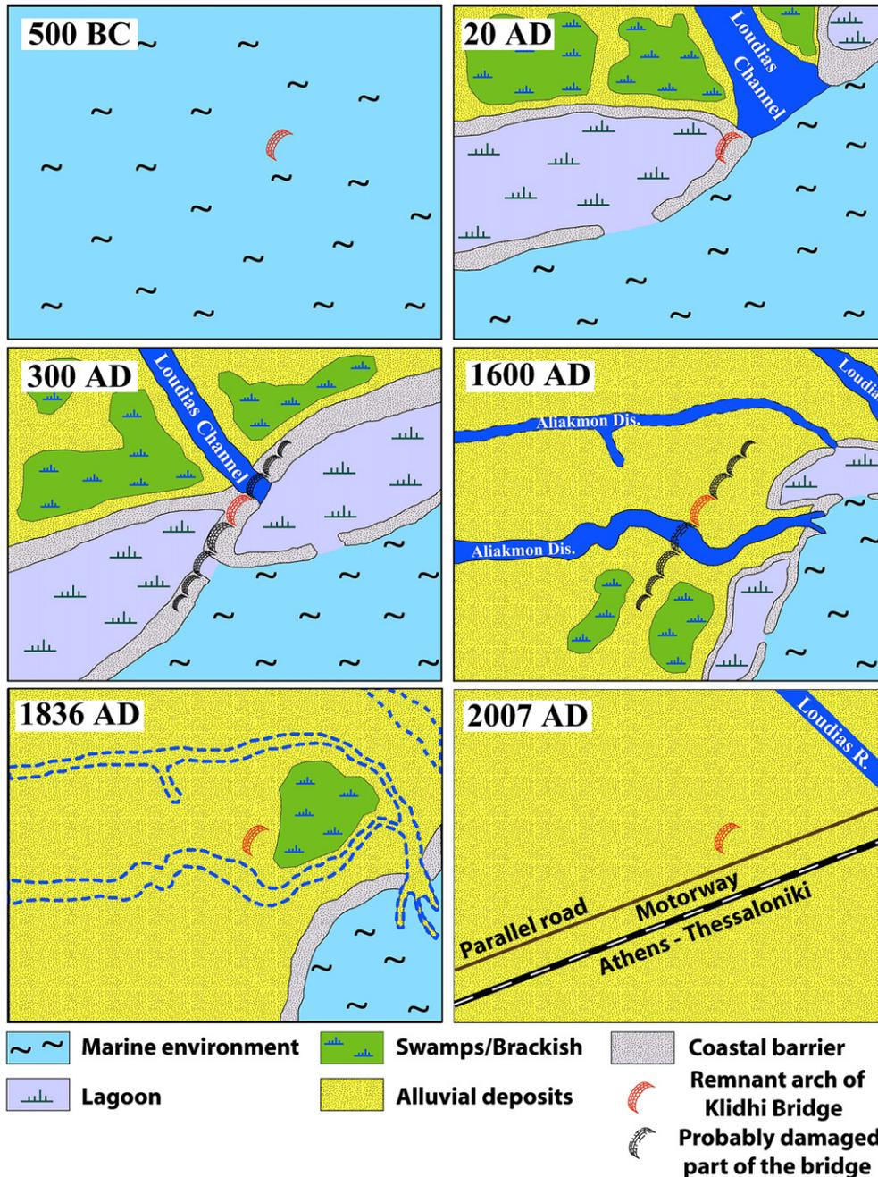
**Fig. 11.** Palaeogeographic reconstruction of the area surrounding the remnant arch of the Klidhi Bridge. The scenario is inferred after combining the results from the palaeoenvironmental study, the historical geography critical analysis and the remote sensing interpretation.
