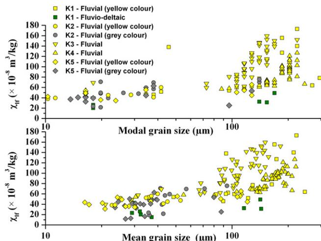
Fig. 7. Magnetic susceptibility measurements vs. grain-size distribution. Upper cartoon: Magnetic susceptibility (Lf) vs. modal index, downer cartoon: magnetic susceptibility (Lf) vs. Mean index
