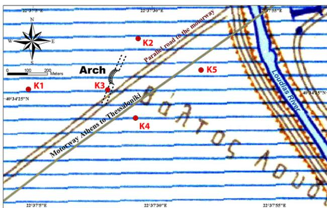
**Fig. 4.** Exact location of the five cores (K1, K2, K3, K4 and K5) drilled in the area surrounding the Ancient Klidhi Bridge. The topographic background corresponds to the topographical map edited by the Hellenic Military Geographical Service (sheet of Plati scaled at 1: 50000).
