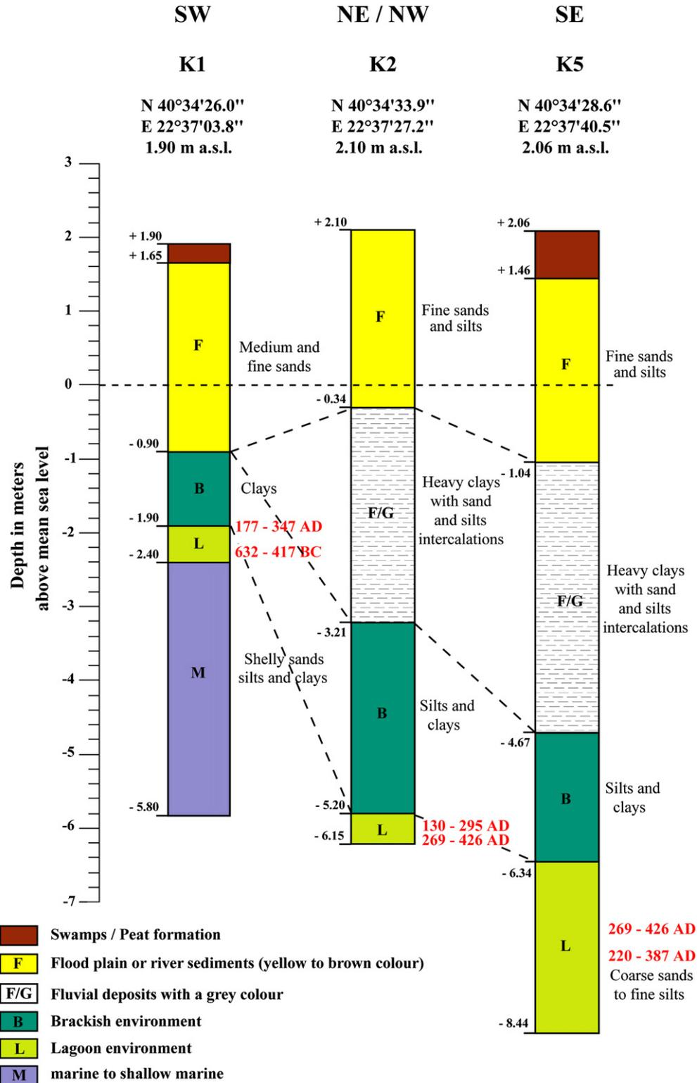
Fig. 9. Cross section using the results derived from cores K1, K2 and K5, the chronostratigraphic sequences are connected together to facilitate a spatial interpretation.
