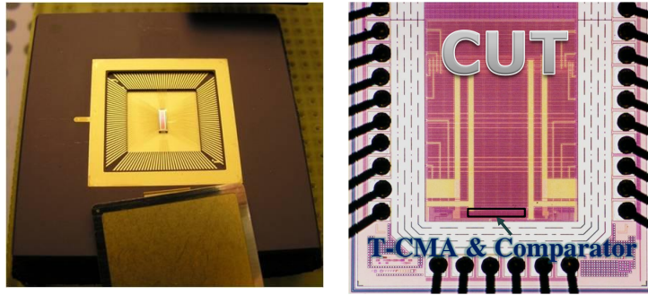
Fig. 12. Fabricated I_{DDQ} test chip and a microphotograph
