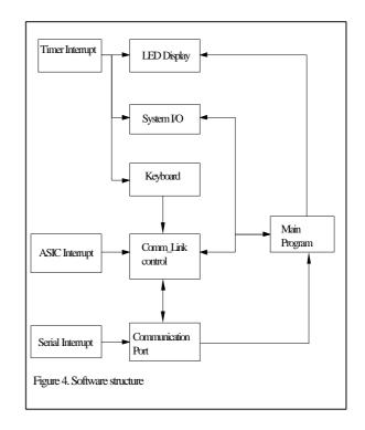
The I/O port is not directly connected to the micro controller. The ASIC has some free I/O pins (totally 16 I/O) to be controlled by the microcontroller. The micro controller controls this I/O ports through the ASIC registers (Table 1). This section of the ASIC is completely irrelevant and independent from the communication link. Thus the keyboard and the LED display are controlled by the micro controller through the ASIC, which is used as an I/O extension of the micro controller.
