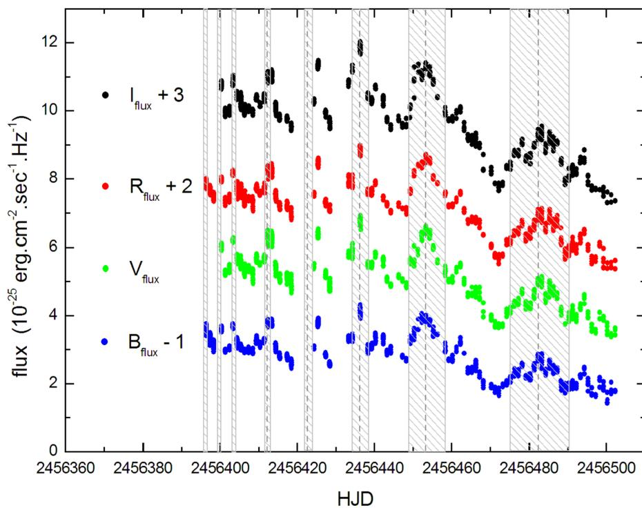
**Figure 1:** The photometric light curves in all optical bands. Gray areas mark the periods of brightness peak, while the width of each box represents the duration of each peak and the dashed line the day of maximum brightness. Note that the (assumed) peak at HJD=2456423.0 is absent, due to bad weather conditions. The observed maximum at HJD=2456425.5 seems to be the secondary peak, following the non-observed one.
