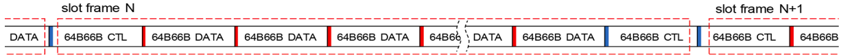
Fig. 11. Slot frame embedded in the sequence of 66-bit blocks of the 10GBASE-R encoding. Slot start and terminate markers are encoded in the type fields of control blocks
