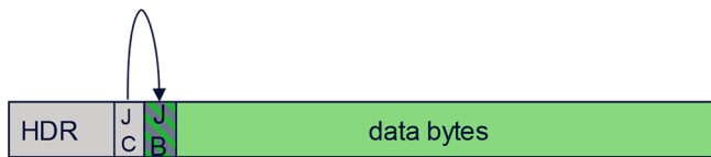
Fig. 12. Rate adaptation by justification control (JC) flag; it assigns the justification byte (JB) to data bytes or not.
