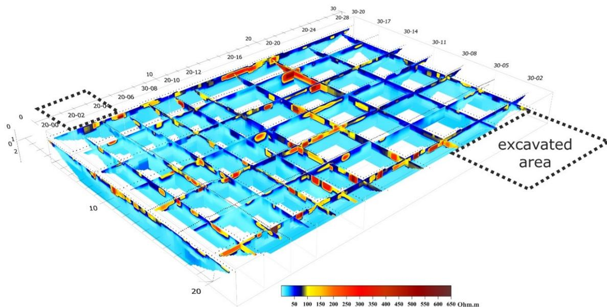
**Figure 3** Fence diagram of the eighteen (18) inverted ERT profiles.
