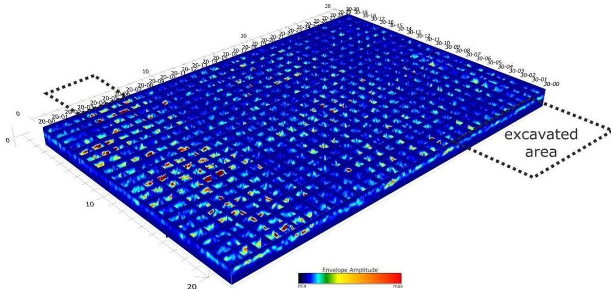
**Figure 2** Fence diagram of the fifty-two (52) GPR profiles.
