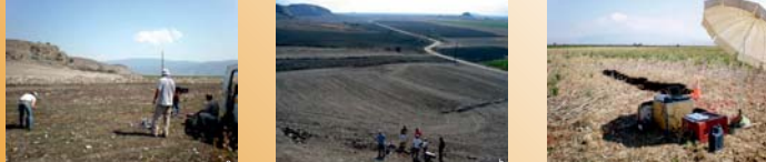
A dense grid of 61 Vertical Electrical Sounding (VES) measurements (Schlumberger array) was designed and carried out covering the entire basin area. The main objective was to investigate the boundaries between the main sediment lithologies and the upper surface of the alpine basement rocks. The geoelectrical data included five (5) "in-situ" resistivity measurements on surface outcrops of the alpine geological formations and fifty six (56) VES measurements at depths around 500 meters. Additionally, data from thirty six (36) unpublished measurements, which were carried out during early 1970's were re-interpreted and re-evaluated, increasing the quantity of data for interpretation, along with a large number of water pumping borehole stratigraphic sections data. The location map of the VES measurements (red dots), in-situ resistivity measurements (green dots) and the boreholes (reverse triangles) the drill sections of which were used for the subsurface basement map, is displayed above. Only the Quaternary outcrops are displayed in colour as all the rest have been removed and replaced by a shaded relief. Purple color shows the areas where the alpine basement was found under the sediments at the depth of investigation. The traces of the sections presented above are also marked. The fieldwork photographs below show VES measurements at Quaternary deposits (a), in-situ VES measurements at alpine basement outcrops (b), as well as Electrical Resistivity Tomographies - not presented in this paper - across observed ground fissures (c).
