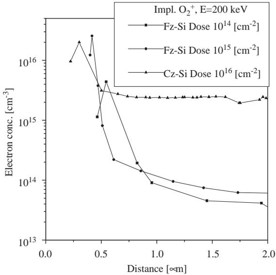
Fig. 2. Electron concentration in Fz-Si and Cz-Si surface layer oxygen implanted with the doses  $10^{14}$ ,  $10^{15}$ , and  $10^{16}$   $\text{cm}^{-2}$  at  $E = 200$  keV.
