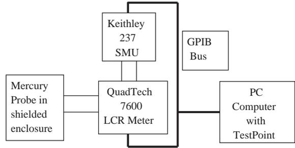
Fig. 1. Block diagram of the electrical measurement setup.
