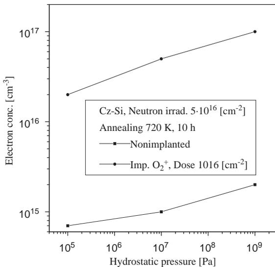
Fig. 5. Electron concentration in the oxygen-implanted and non-implanted Cz-Si surface layer after neutron irradiation as a function of hydrostatic pressure applied during annealing at 720 K for 10 h.
