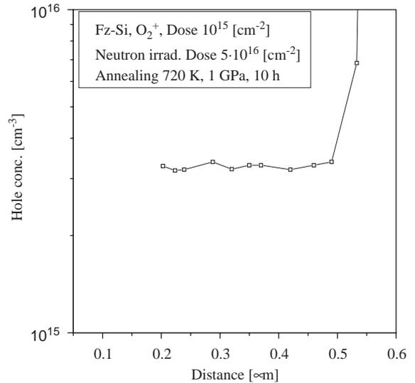
Fig. 4. Hole concentration in the oxygen-implanted Fz-Si surface layer after neutron irradiation and annealing at 720 K, 1 GPa for 10 h.
