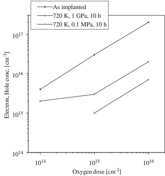
Fig. 3. Electron and hole concentration in the Fz-Si surface layer as a function of implanted dose.
