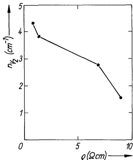
Fig. 2. The introduction rate of  $V_2$  created during irradiation in the primary collision process as a function of specific resistivity
