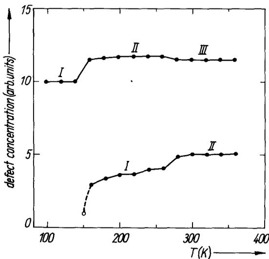
Fig. 1. The evolution of A-centers (lower curve) and  $V_2$  (upper curve) after irradiation at 80 K
