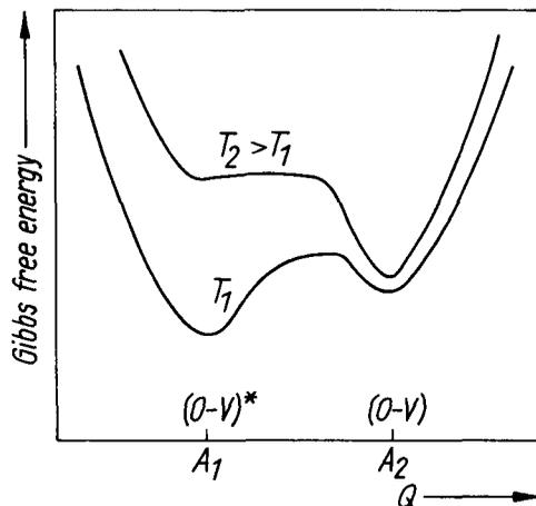
Fig. 3. A rough schematic diagram of the Gibbs free energy as a function of a general coordinate  $Q$ , suggested for the A-center
