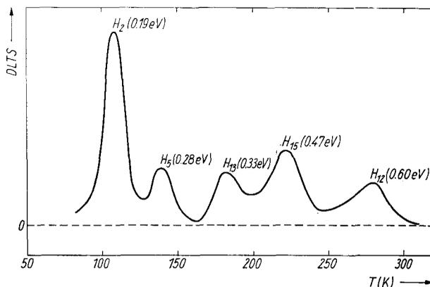
Fig. 1. The DLTS spectrum of float-zone Si:B,  $p = (6.4 - 7.4 \Omega \text{ cm})$ , 1.5 MeV electron irradiated at 80 K to a dose of  $\approx 1.7 \times 10^{16} \text{ e}^-/\text{cm}^2$  and a beam current of  $\approx 0.15 \mu\text{A}/\text{cm}^2$ , after an anneal at 470 K for 90 min (rate window =  $5 \text{ s}^{-1}$ )
