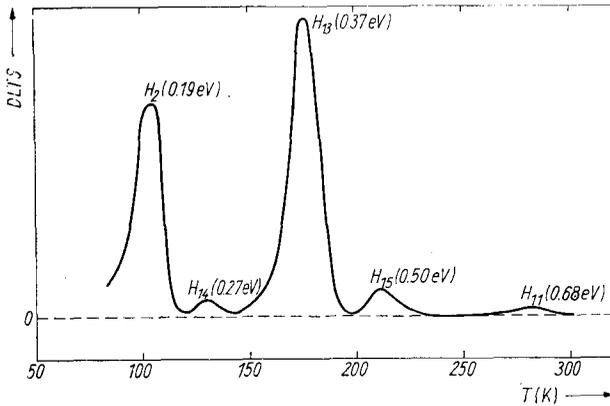
Fig. 2. The DLTS spectrum of pulled Si:B,  $p = (3 - 5 \Omega \text{ cm})$ , 1.5 MeV electron irradiated at 80 K to a dose of  $\approx 3.5 \times 10^{16} \text{ e}^-/\text{cm}^2$  and a beam current of  $\approx 0.33 \mu\text{A}/\text{cm}^2$ , after an anneal at 470 K for 90 min (rate window =  $5 \text{ s}^{-1}$ )
