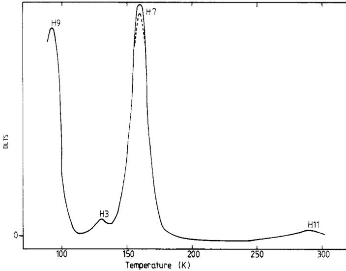
**Figure 3.** DLTS signals (in arbitrary units) for the specimen after irradiation and annealing at 315 K for 1 h (rate window  $0.4 \text{ s}^{-1}$ ). The MCTS signal was unchanged from that for figure 2, with no features between 215 and 315 K.
