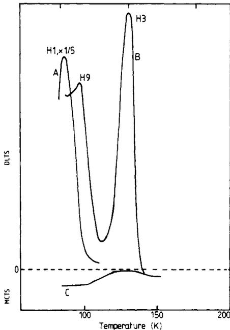
**Figure 1.** DLTS and MCTS signals (both given in arbitrary units) for the specimen after irradiation at about 80 K. (A) Rate window  $2500 \text{ s}^{-1}$  (DLTS). (B) Rate window  $0.4 \text{ s}^{-1}$  (DLTS). (C) Rate window  $2 \text{ s}^{-1}$  (MCTS).
