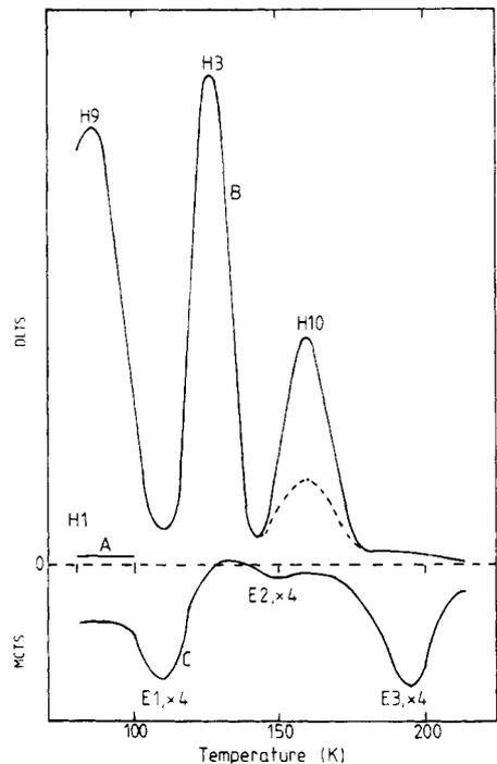
**Figure 2.** DLTS and MCTS signals (both given in arbitrary units) for the specimen after irradiation and annealing at 215 K for 30 min. (A) Rate window  $2500 \text{ s}^{-1}$  (DLTS). (B) Rate window  $0.4 \text{ s}^{-1}$  (DLTS): full curve, after zero-bias anneal; broken curve, after anneal under reverse bias of 5 V. (C) Rate window  $2 \text{ s}^{-1}$  (MCTS).
