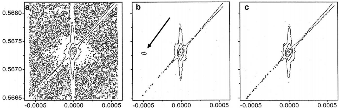
Fig. 4. 004 XRRSMs of Cz-Si:Ge processed for 5 h at 1270 K under  $10^5$  Pa (a), 1.1 GPa (b) and, sequentially, for 5 h under 1.1 GPa at 1070 K and for 5 h at 1270 K under 1.1 GPa (c).
