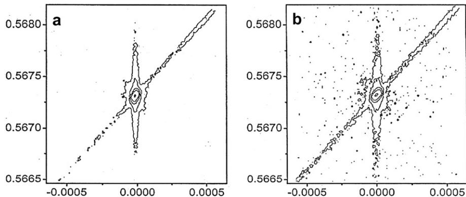
Fig. 6. 004 XRRSMs of Cz-Si:Ge processed for 5 h at 1400 K under  $10^5$  Pa (a) and 1.1 GPa (b).
