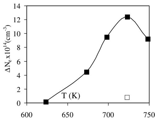
Fig. 1. Dependence of  $N_e$  ( $N_e = N_{\text{HT-HP}} - N_i$ , where  $N_{\text{HT-HP}}$  – concentration of electrons after processing at HT–HP and  $N_i$  – initial concentration of carriers) on processing temperature for Cz-Si:Ge samples treated for 10 h at 625–750 K under  $\text{HP} = 1.1\text{--}1.2 \text{ GPa}$  (■).  $N_e$  for Cz-Si:Ge processed for 10 h at 723 K under  $10^5 \text{ Pa}$  is indicated (empty mark, □).
