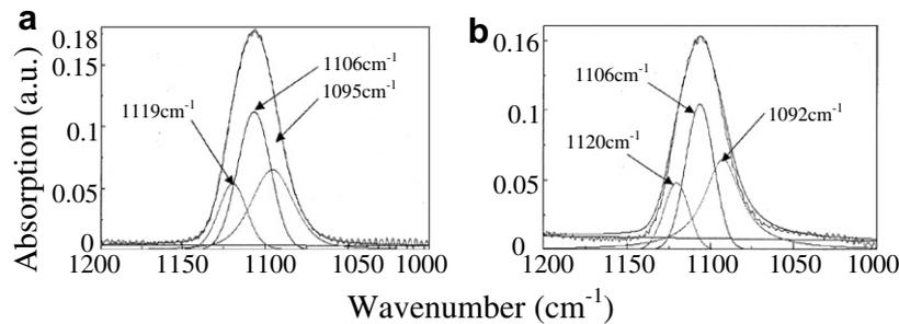
Fig. 5. Deconvolution of IR absorption of Cz-Si:Ge processed for 5 h at 1400 K under  $10^5$  Pa (a) and 1.1 GPa (b).
