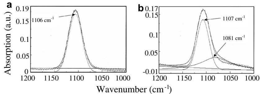
Fig. 2. Deconvolution of IR absorption of Cz-Si:Ge treated for 10 h under 1.1 GPa at 723 K (a) and 923 K (b).
