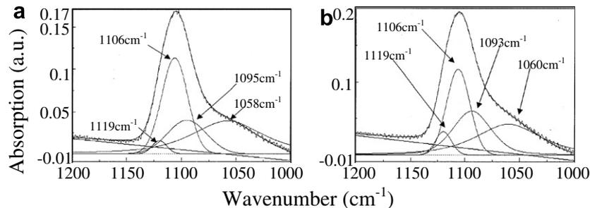
Fig. 3. Deconvolution of IR absorption of Cz-Si:Ge processed for 5 h at 1270 K under 10<sup>5</sup> Pa (a) and 1.1 GPa (b).
