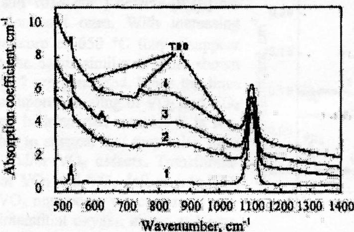
Fig. 1. Fragments of absorption spectra at 300 K of Cz-Si samples in as-grown state (1) and after treatments at 450 °C for 60 h (2), 120 h (3) and 240 h (4)
