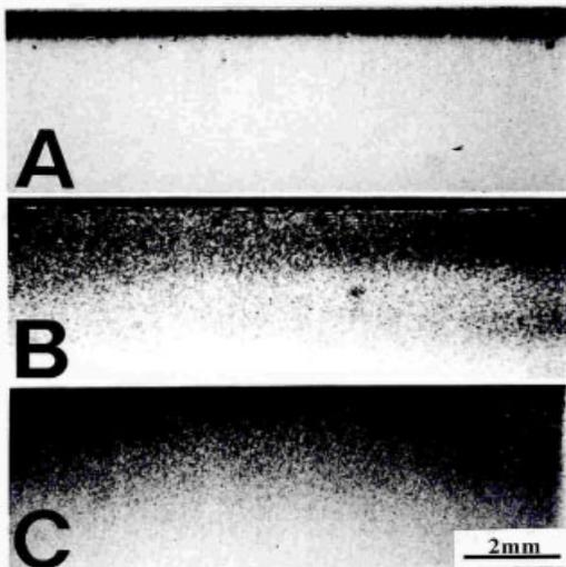
**Fig. 1** Bragg case synchrotron white beam topographs of R (A) and NI samples (B and C) annealed / treated at 1270 K under  $10^5 \text{ Pa}$  (A and B) and 1.1 GPa (C).
