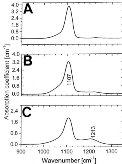
**Fig. 3** FTIR absorption spectra taken at 300 K for R (A) and NI (B and C) samples, annealed / treated at 1270 K under  $10^5\text{ Pa}$  (A and B) and 1.1 GPa (C).
