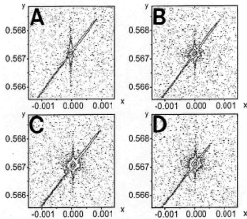
**Fig. 2** XRRSMs of R (A and C) and NI (B and D) samples processed at 1270 K under  $10^5\text{ Pa}$  (A and B) and 1.1 GPa (C and D). The axes are marked in  $\lambda/2d$  units ( $\lambda$  - wavelength,  $d$  - inter-planar distance).
