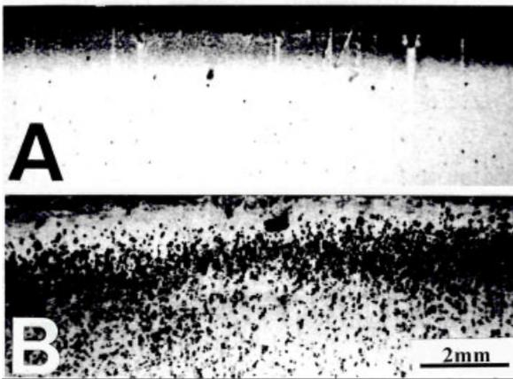
**Fig. 5** Bragg-case white beam topographs of R (A) and NI (B) samples annealed / treated at 1400 K under  $10^5$  Pa (A) and 1.1 GPa (C).
