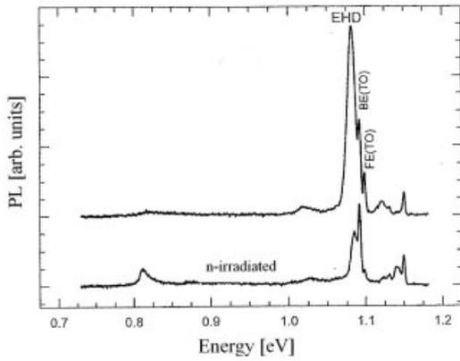
**Fig. 4** PL spectra of reference (non-marked) and neutron – irradiated samples treated at 1270 K under 1.1 GPa. EHD (electron – hole droplet) means the recombination related to electron – hole droplet; BE(TO) and FE(TO) – the transverse optical phonon replicas of bound exciton and of free exciton recombination, respectively.
