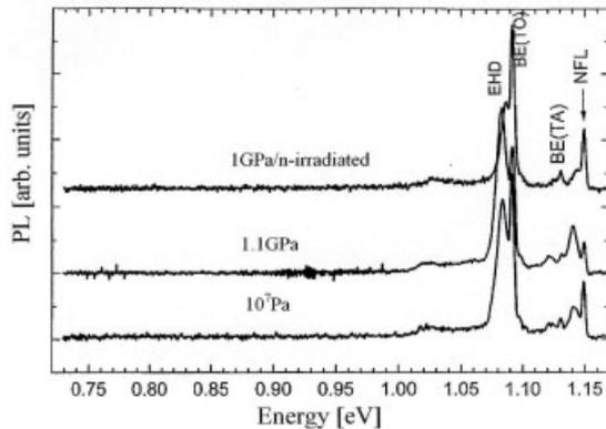
**Fig. 7** PL spectra of reference R and neutron – irradiated NI samples annealed / treated at 1400 K under  $10^5$  Pa and 1.1 GPa. BE(TA) means the recombination of transverse acoustic phonon replica of boron bound exciton and NFL - the non – fonon recombination of excitons.
