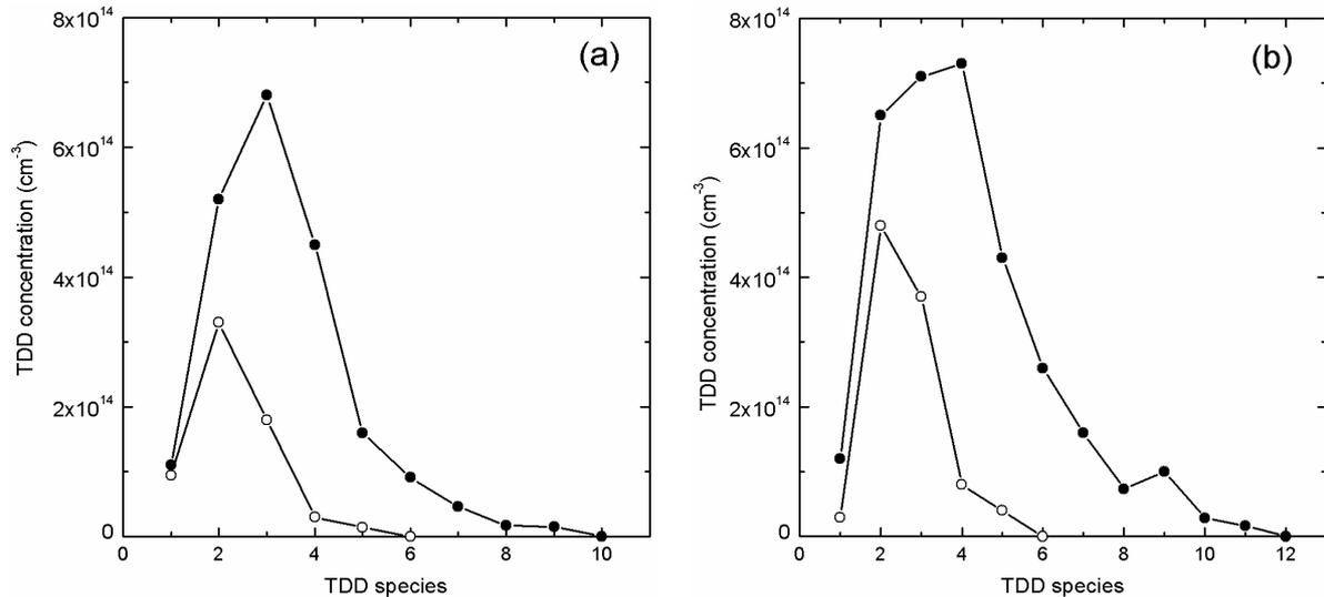
**Fig. 3** TDD distributions in the heat-treated Cz-Si with different initial oxygen concentrations  $N_{oxy}^0$ : (a)  $6.0 \cdot 10^{17} \text{ cm}^{-3}$  and (b)  $9.5 \cdot 10^{17} \text{ cm}^{-3}$ . Heat treatment at  $T = 450^\circ \text{C}$  for  $t = 2$  h (open circles) and 10 h (solid circles) under a hydrostatic pressure  $P = 1.2 \text{ GPa}$ .
