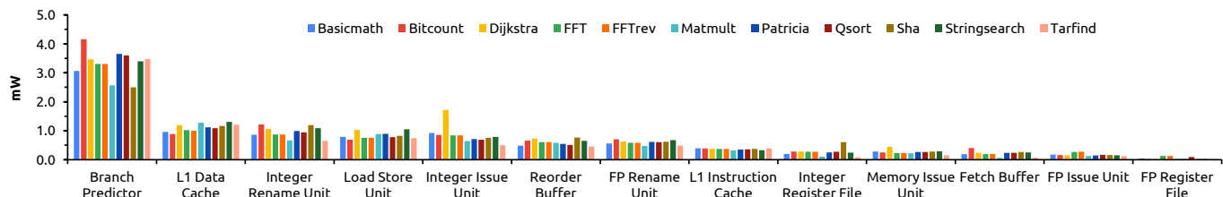
Fig. 5. Power consumption per hardware structure for the MediumBoom across all eleven benchmarks.
