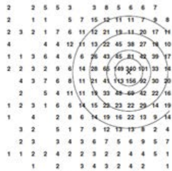
Fig. 8.13. Map of an air shower in a 196 detector array on a 15 m grid. The densities from (8.18) fluctuate with a Gaussian distribution with \sigma = \sqrt{\bar{\rho}} . Because of that some detectors do not trigger.
