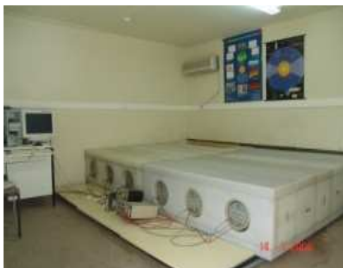
Figure 1. Infrastructure of registration system of ANeMoS consisting of 6NM-64 counters.
