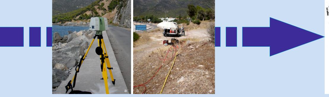
Field work data acquisition by surveying with the terrestrial laser scanner at the station SG-2 (a) and geophysical tomography along the ERT-1 section above the debris formation (b). The fault scarp is visible at the top right of figure (a).
