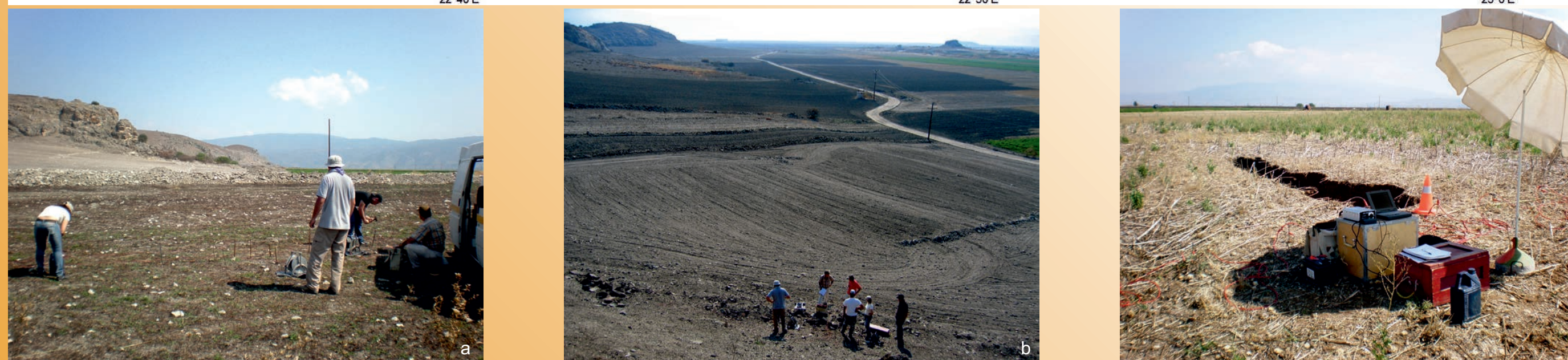
A dense grid of 61 Vertical Electrical Sounding (VES) measurements (Schlumberger array) was designed and carried out covering the entire basin area. The main objective was to investigate the boundaries between the main sediment lithologies and the upper surface of the alpine basement rocks. The geoelectrical data included five (5) "in-situ" resistivity measurements on surface outcrops of the alpine geological formations and fifty six (56) VES measurements at depths around 500 meters. Additionally, data from thirty six (36) unpublished measurements, which were carried out during early 1970's were re-interpreted and re-evaluated, increasing the quantity of data for interpretation, along with a large number of water pumping borehole stratigraphic sections data.
