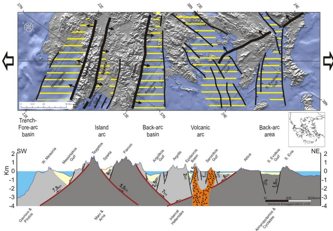
Fig. 2: In this vertically exaggerated (x10) SW-NE section across the Southern Hellenides the post-nappestacking extensional structures are indicated.
