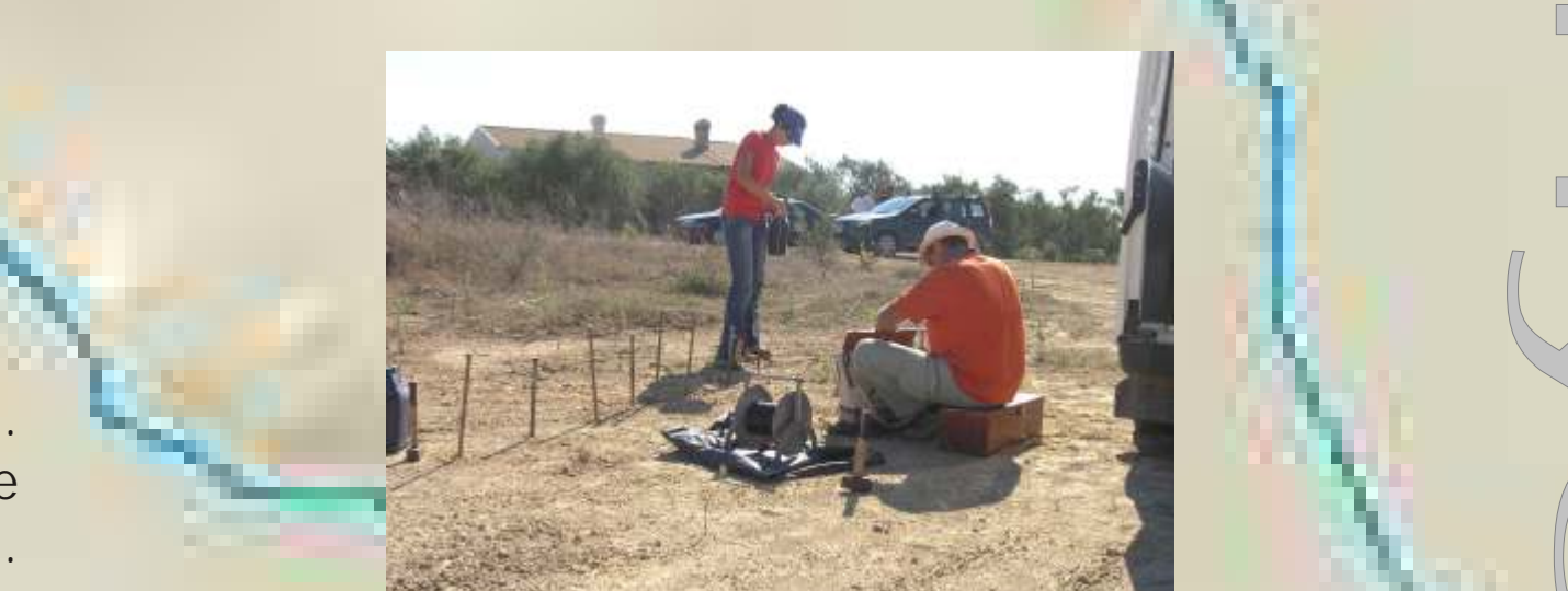
Figure 18. Five in situ soundings were carried out at outcrops of the post alpine formations by applying the Schlumberger array configuration.
