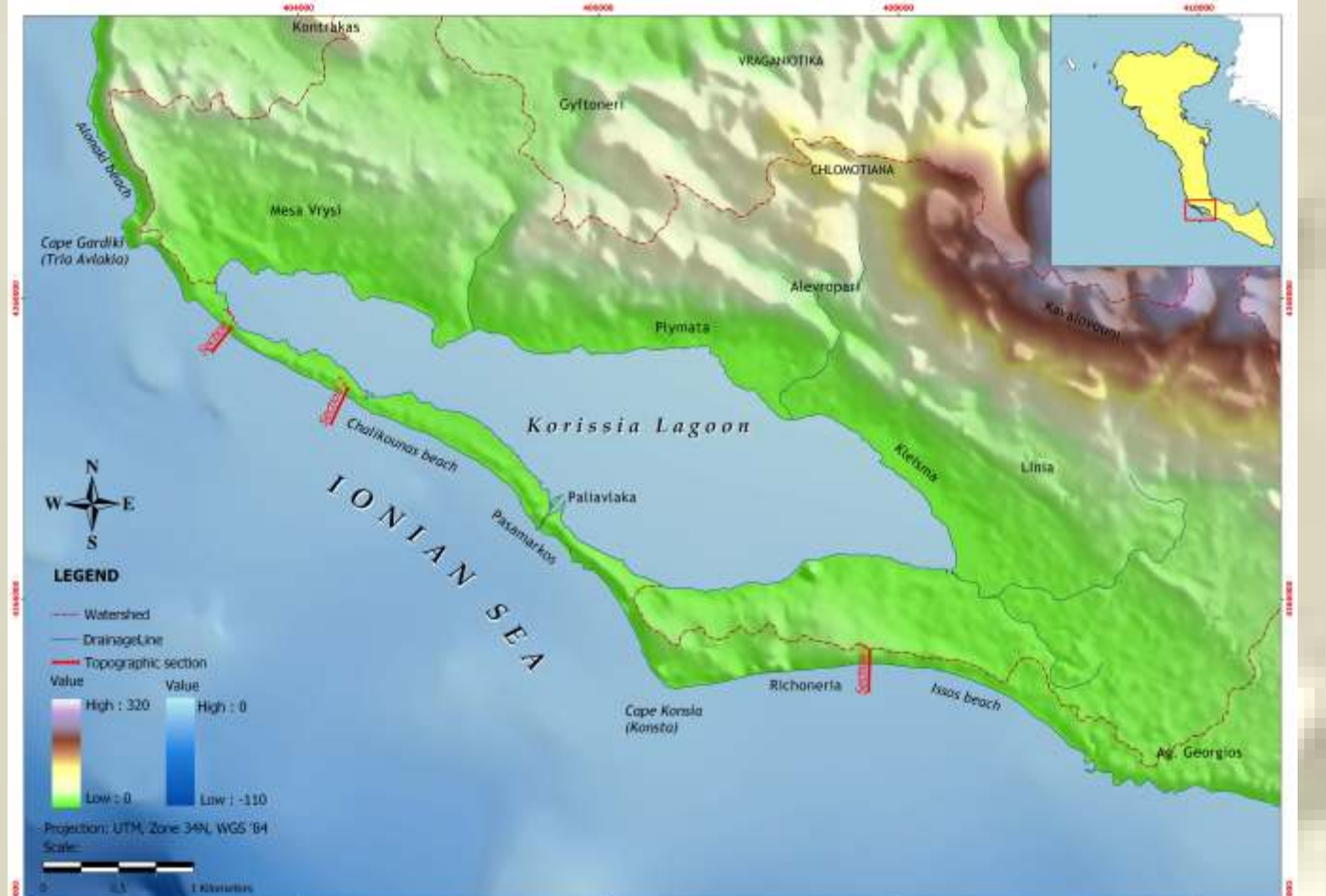
Figure 2. Elevation map and shaded relief of the study area created by the interpretation of high resolution digital elevation model. The main channels of the drainage network are also shown in the watershed around the lake area. The three high detailed topographic surveys are also marked in red.
