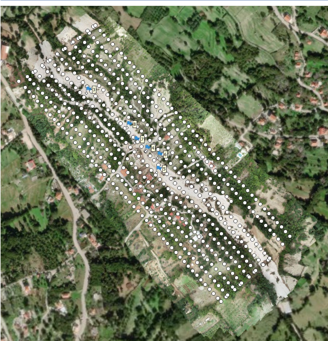
Figure 1. Flight plan and image locations (533 images).
