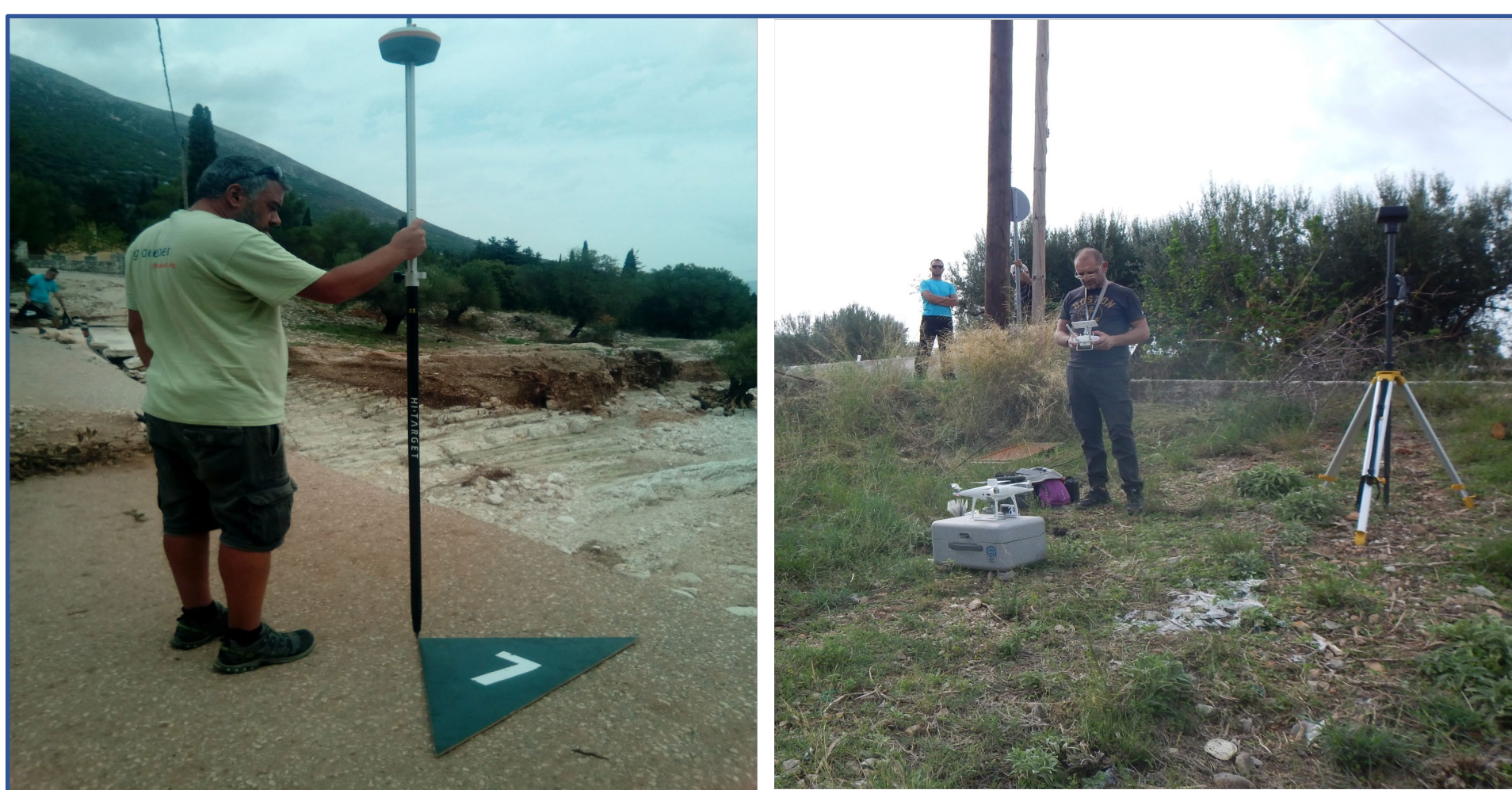
Figure 2. Set up of GCP points and DJI Phantom 4 RTK (Left and Right).
