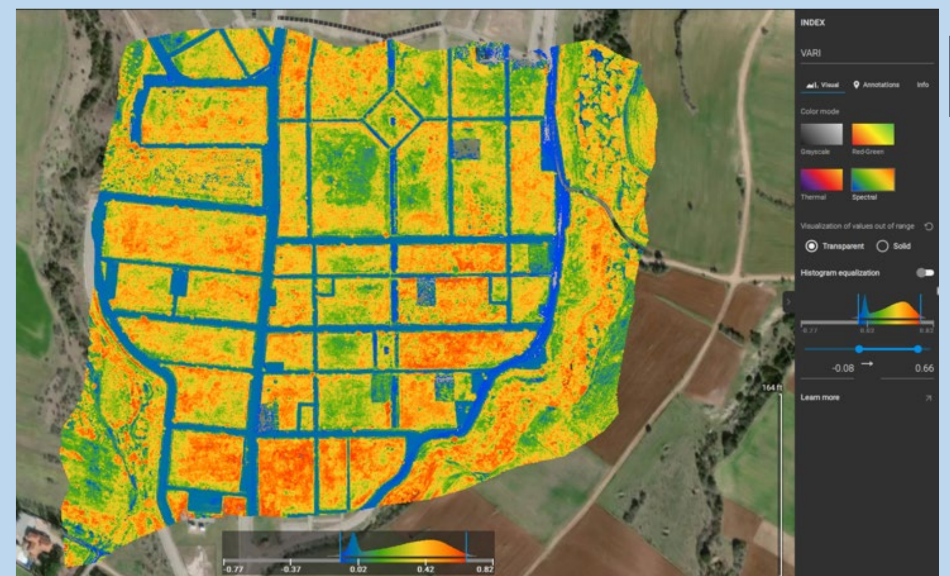
Figure 6. Visible Atmospherically Resistant Index (VARI) index is perfect for RGB or color images since it works with the whole visible segment of the electromagnetic spectrum (comprising red, green, and blue color bands). Its specific task is to enhance vegetation under strong atmospheric impact while smoothing illumination variations.
