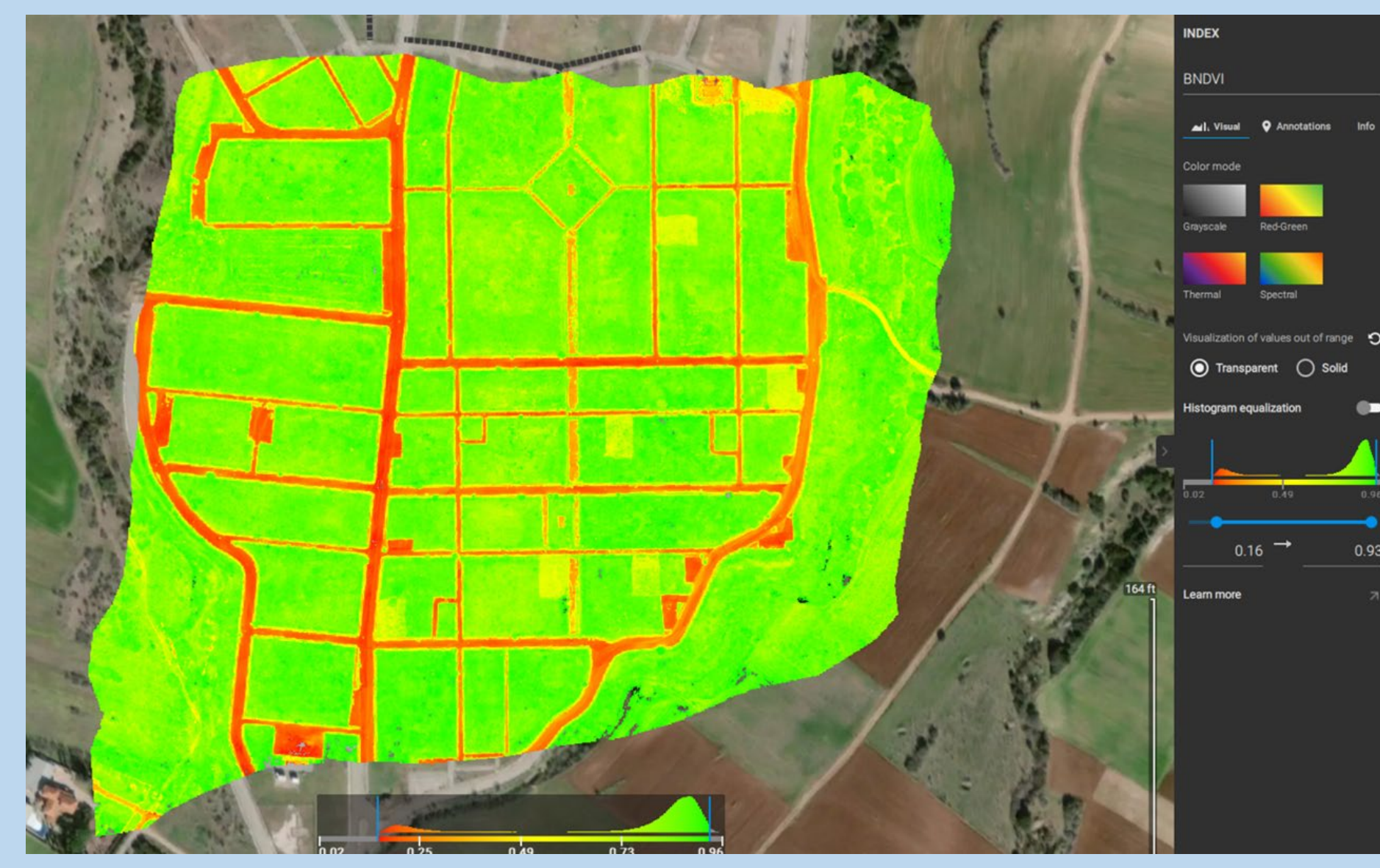
Figure 7. Blue Normalized Difference Vegetation Index (BNDVI) is much similar to NDVI except that instead of the red wavelength of the spectrum it uses the blue wavelength of the spectrum (NIR-Blue)/(NIR+Blue). This is an indicator of for areas that are sensitive to chlorophyll content.
