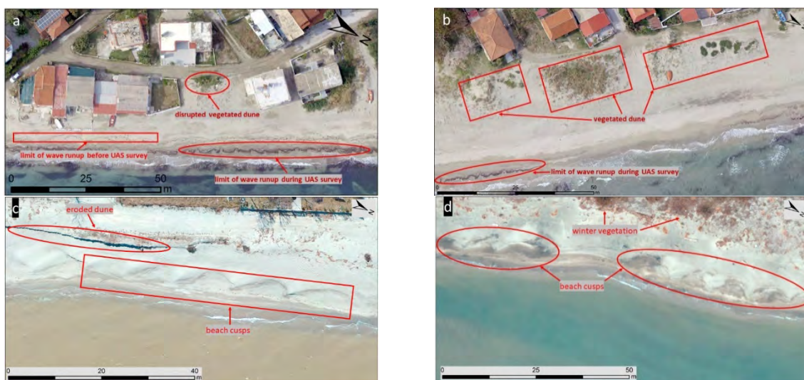
Figure 3 The potential of UAS surveys in coastal monitoring: a) old/contemporary wave runup level and disrupted dune at a part of Nea Mesagkala beach characterized by shoreline retreat during whole monitoring period, b) vegetated dunes and wave runup in Nea Mesagkala, c) beach cusps and eroded dune in Alexandrini
