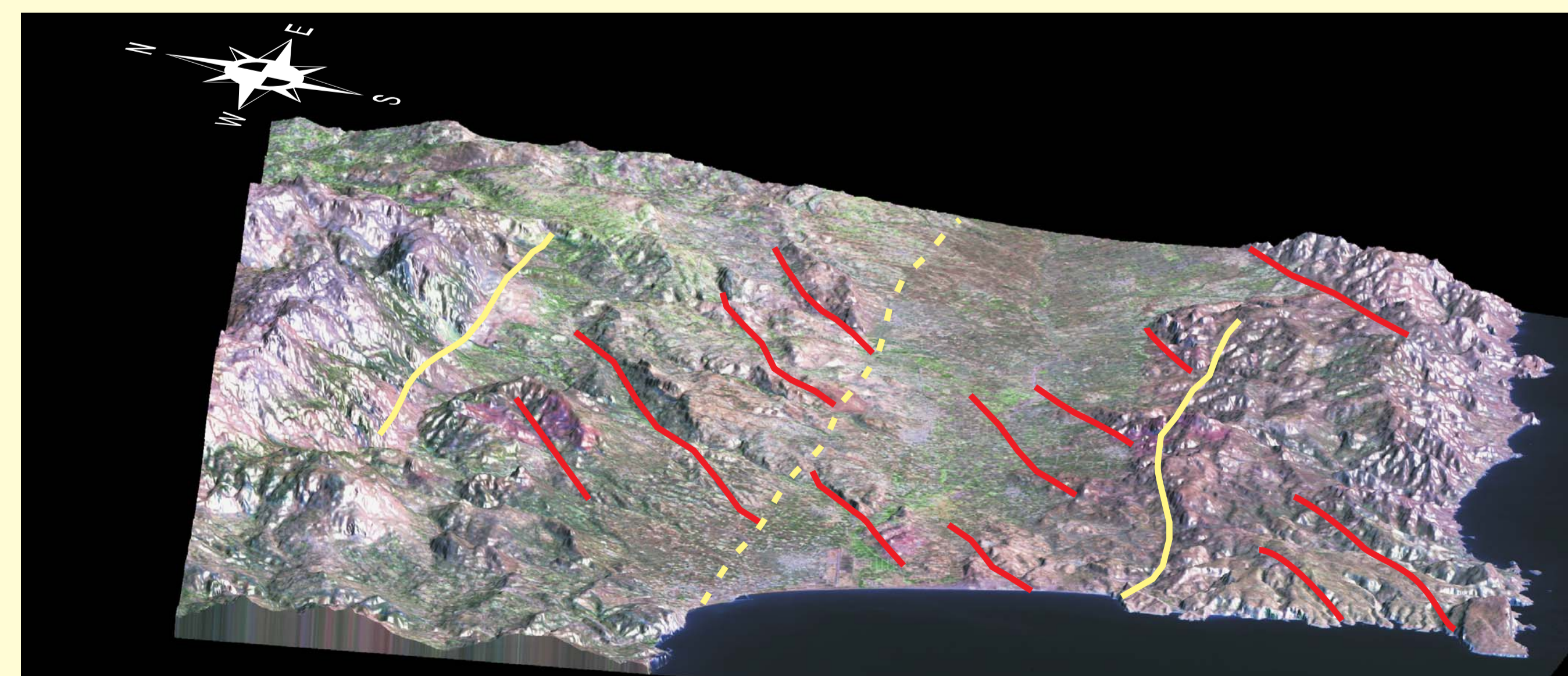
Three dimensional perspective model of the Messara basin. The shaded relief - satellite image combination was further processed by means of artificial illumination. This figure allows the easy identification of co-existing E-W (yellow) and NE-SW (red) neotectonic structures.
