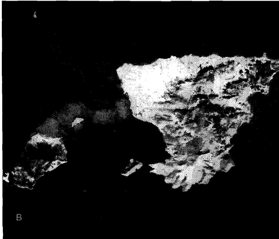
**Fig. 4:** Landsat 5 TM, band 1, geometrically corrected, subscene of the study area, before (A) and after (B) processing. In the image B is emphasized the well recorded reflectance properties of the bottom, between Agistri and Aegina islands.
