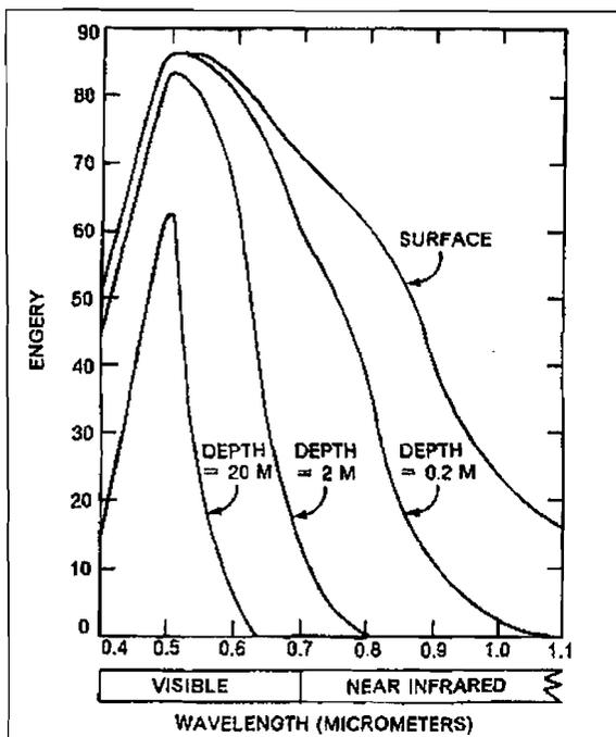
**Fig. 1:** Spectral characteristics of sunlight as it penetrates a clear water body. Near the surface the curve resembles the spectrum of solar radiation, but the water body increasingly influences the spectral composition of the light as depth increases. At a depth of 20 meters no infrared radiation is present as the water body is an effective absorber of these longer wavelengths. From Moore (1978).
