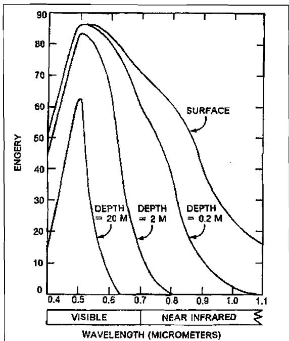
**Fig. 1:** Spectral characteristics of sunlight as it penetrates a clear water body. Near the surface the curve resembles the spectrum of solar radiation, but the water body increasingly influences the spectral composition of the light as depth increases. At a depth of 20 meters no infrared radiation is present as the water body is an effective absorber of these longer wavelengths. From Moore (1978).
