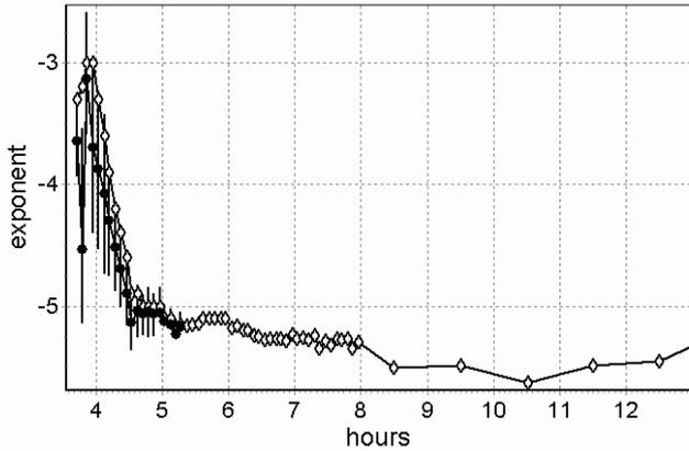
**Fig. 8.** Behavior of the power law index (exponent) for isotropic (starting from the 16th 5-min interval), and anisotropic (the first 15 five-min intervals) models, together with mean flux, averaged by all directions (for 1 GeV energy).
