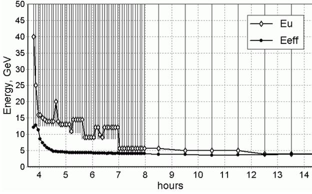
**Fig. 10.** Behavior of upper limited energy  $E_u$  of solar CR (diamonds) and their effective energy  $E_{eff}$  from neutron monitor network registration.
