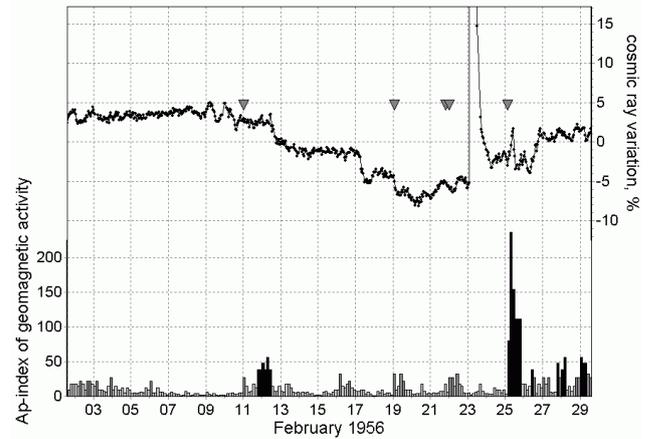
**Fig. 2.** Counting rate variations at Climax neutron monitor and Ap index of geomagnetic activity in February 1956. Great fluxes on 23 February are not plotted. Triangles at the top of the figure correspond to the SSC.
