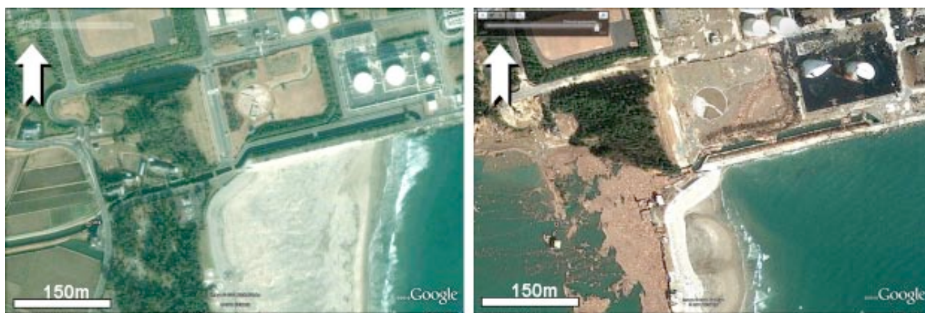
Fig. 1. Minamisoma coastal area (Fukushima prefecture). Total erosion of shoreline, total deforestation of vegetation in low lying area, submergence of low lying cultivated area into a lagoon-like form, functioning as a retention pond for water backwash after the tsunami. Debris accumulated behind the road embankment and into the newly formed lagoon. Treatment Plant in nearby industry is devastated, as much as the tanks which may also have been set on fire during the disaster.
