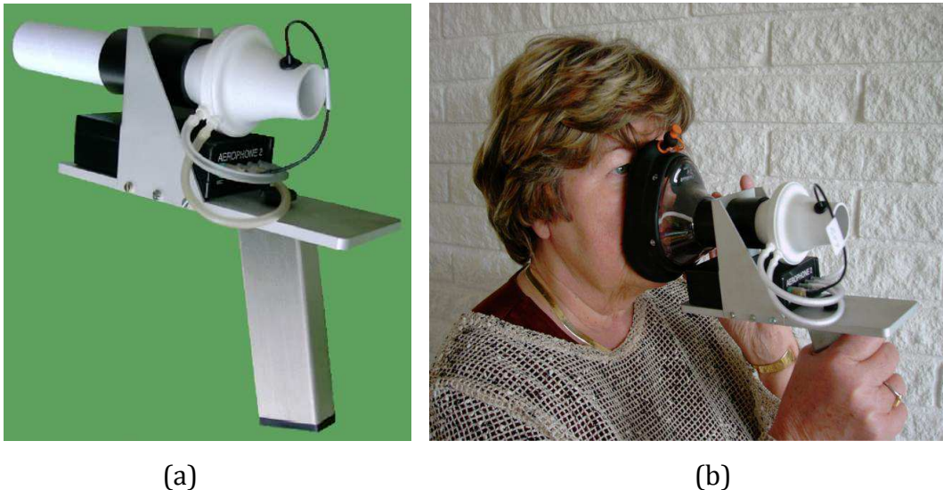
Figure 2. The Aerophone II apparatus (a) and its usage for the aerodynamic measurements of voice (b).
