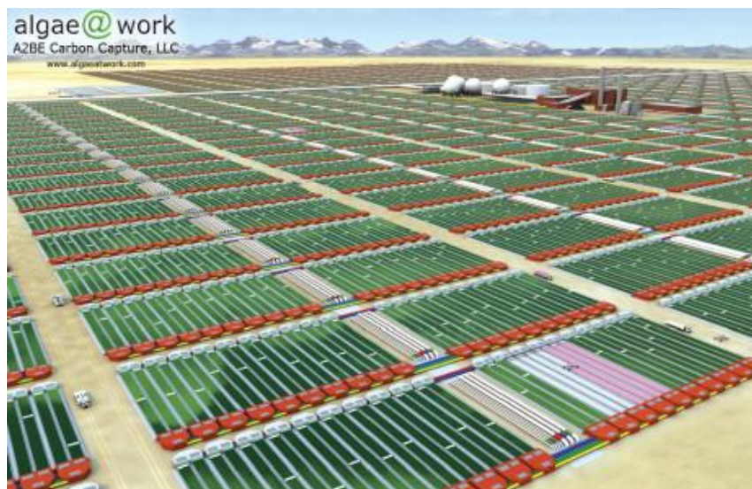
Figure 9. Farms of photosynthetic algae can be used to capture carbon dioxide from the air and with the sun's rays convert it into biomass and heat.
