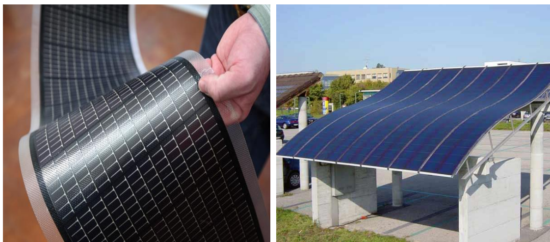
Figure 12. Thin film photovoltaic cells are made from materials that absorb sunlight very strongly. While a crystalline silicon solar cell is 0.1-0.2 mm thick, thin film cells are about 0.01 mm thick. That thinness means it can be manufactured with relatively inexpensive roll-to-roll fabrication techniques. It also means thin film solar materials are light and flexible.
