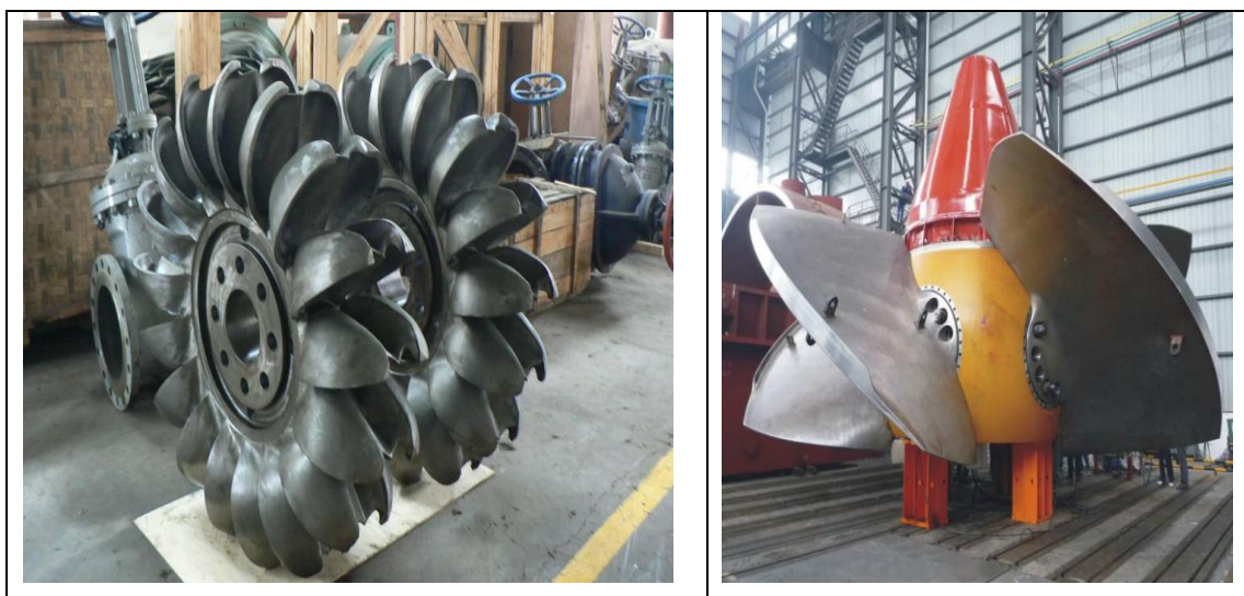
Figure 16. Modern hydropower turbines are constructed from steel, or new alloys of tungsten carbide, or fiber-reinforced composites to withstand high pressures and resist corrosion from sediments.
