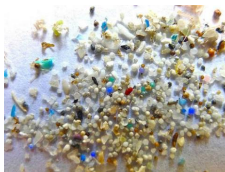
Figure 9. The degradation of plastic items produce a vast number of small sized plastic beads, microplastics (<1 mm) that spread in the sand in the sea beds.
