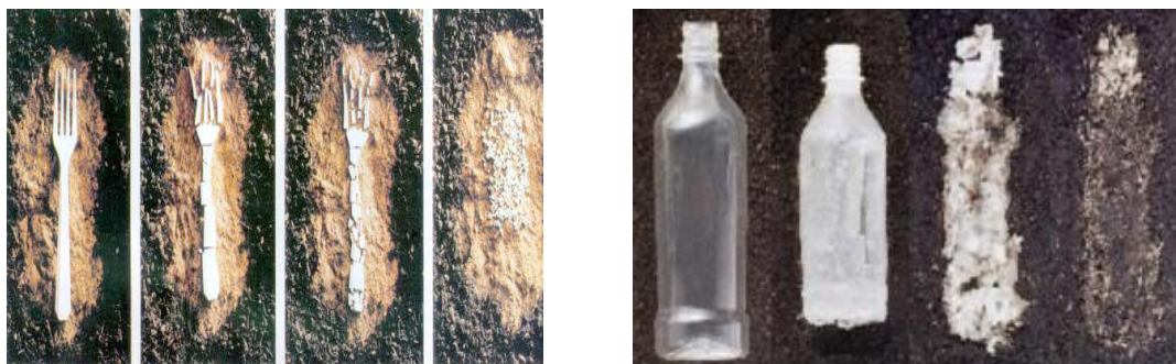
Figure 8. Biodegradable plastic materials can be “degradable” but still last for a long time in the environment. Hydrolytic degradation has certain environmental requirements, a material may degrade readily in one environment and be long-lasting in another.
