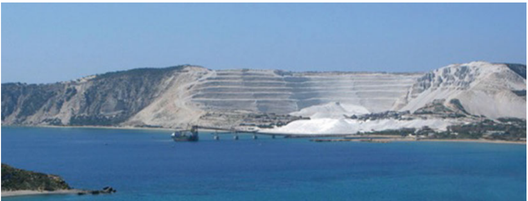
Fig. 2.28 The Yali pumice deposits are exposed as 60–100 m high cliffs, dipping 10^\circ towards SW and comprise a minimum volume 0.3 \text{ km}^3 , with the base and submarine portion unknown. The deposits are dissected by normal
