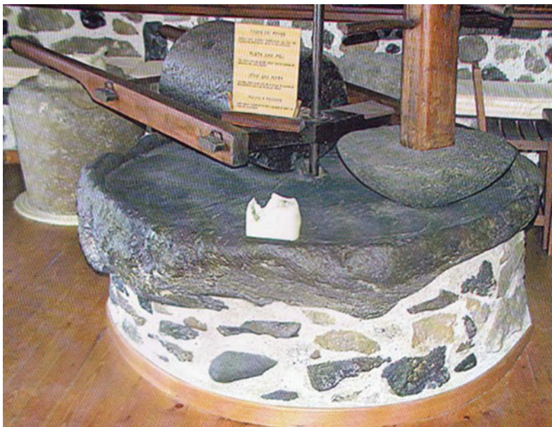
Fig. 1.7 Millstone exhibition in the “Liotridia” (“oil pressing”) hotel, a former olive oil pressing establishment at the waterfront in Mandraki. The millstone dish and barrel are carved out of andesite lava from idle quarries at the seaside east of Mandraki; in background a grey
