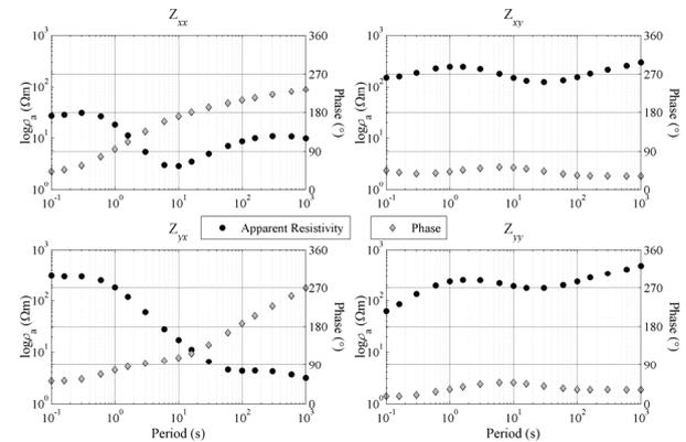
Figure 1. The noise-free almost exact impedance tensor “observed” at *Site 4* of the 2-D anisotropic model of Heise and Pous (2003).
