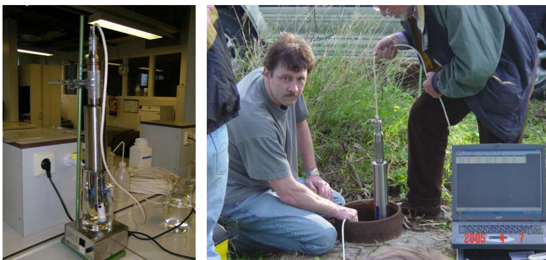
Figure 1. Left: The probe complete with ISE's during calibration with standard solutions. Right: The probe while inserted in a well. In this case, the system is configured for single-site measurements and in addition to the probe it comprises a data logger and a laptop or palmtop computer to control data acquisition and storage.
