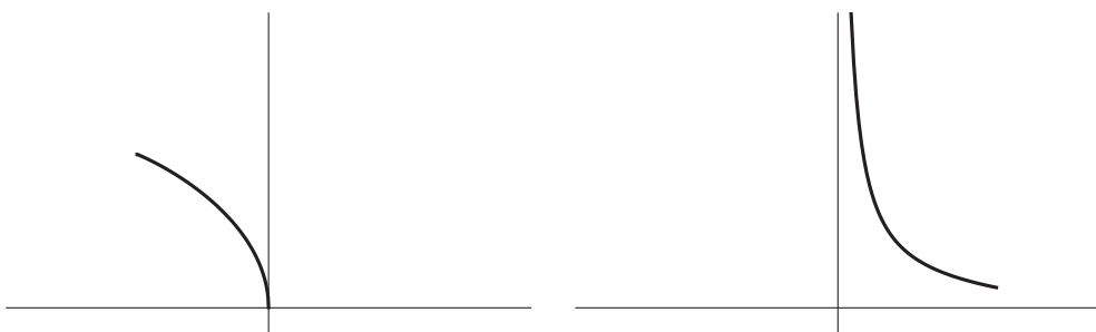
Figure 4. The enveloped curve FG of Newton's construction in the cases y(x) = \sqrt{x} (left) and y(x) = x^2 (right).
